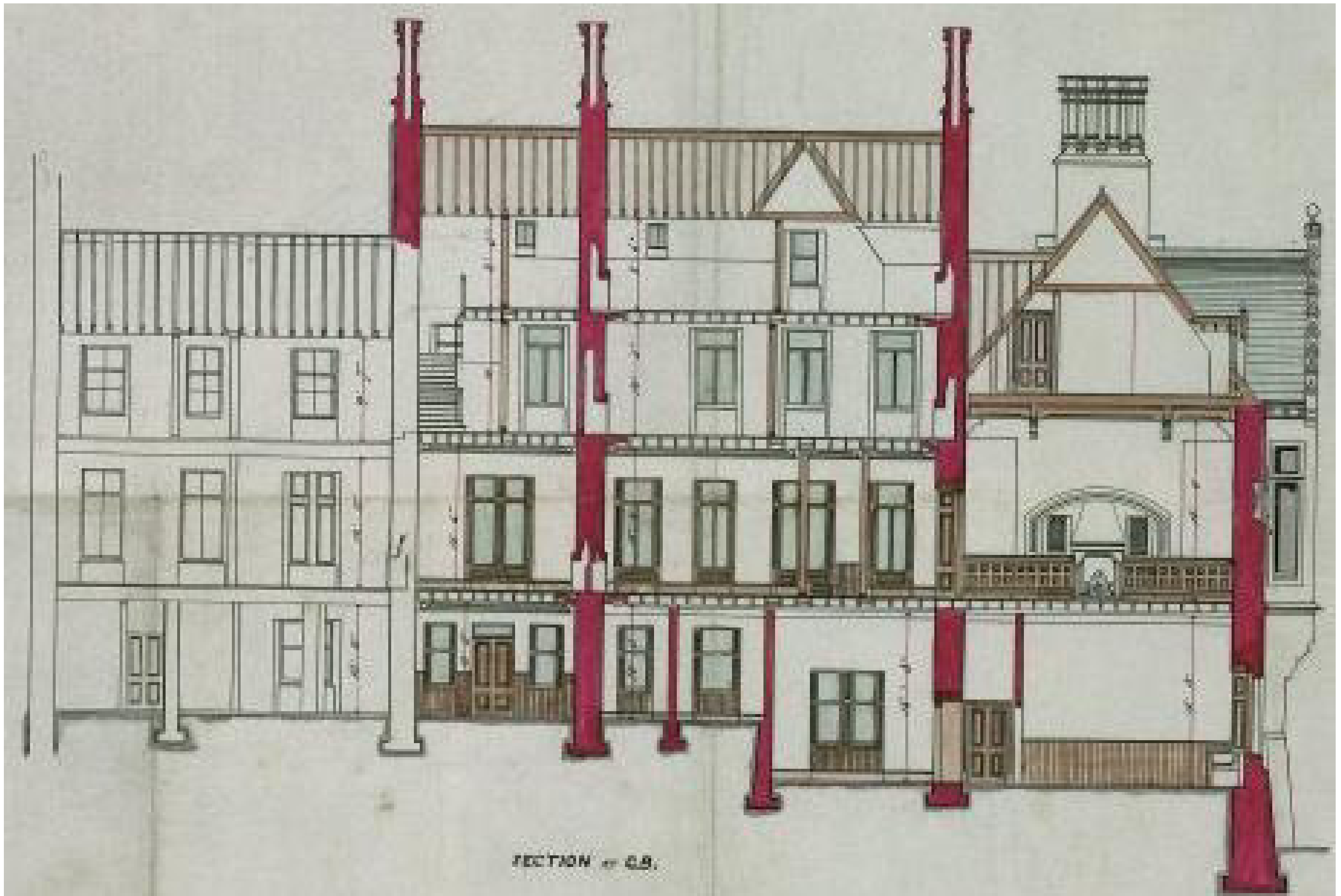
Illus 87 1882 W-E section showing Phase 1 house (left) with addition (right) and chimneys (in red); window W18 is on the extreme right and arched fireplace 15 to the left of W18 (copyright RCAHMS)
