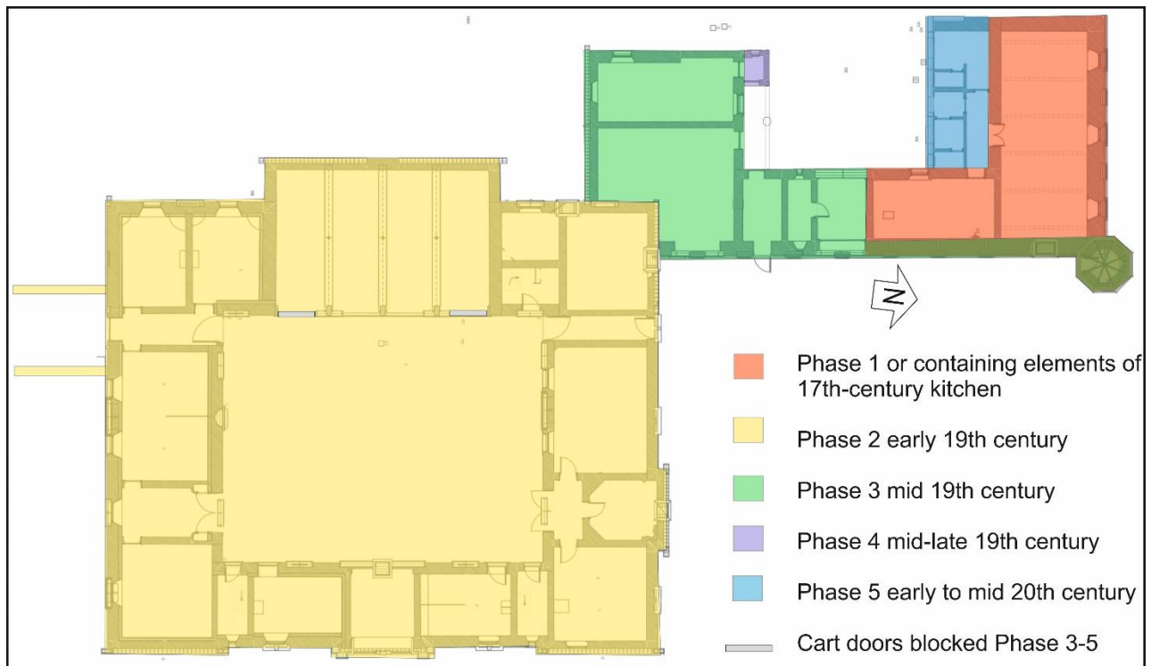
Illus 54 Phase plan showing main phases of developments of the buildings (copyright Building Workshop)
