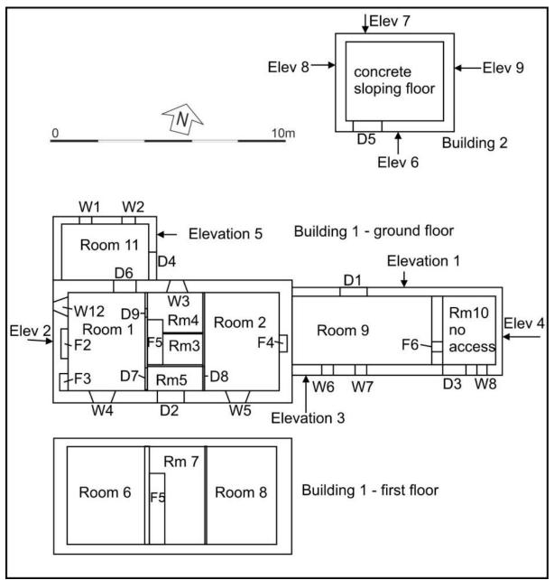
Illus 2 Plan of croft including first floor annotated with numbers used in this survey
