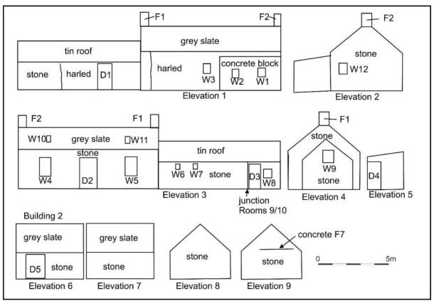
Illus 3 Elevations of croft including first floor annotated with numbers used in this survey
