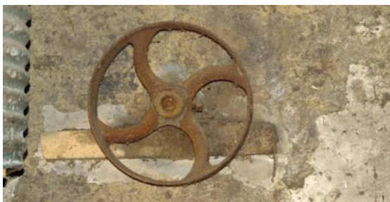
Fig 19 Barn interior S wall drive pulley
