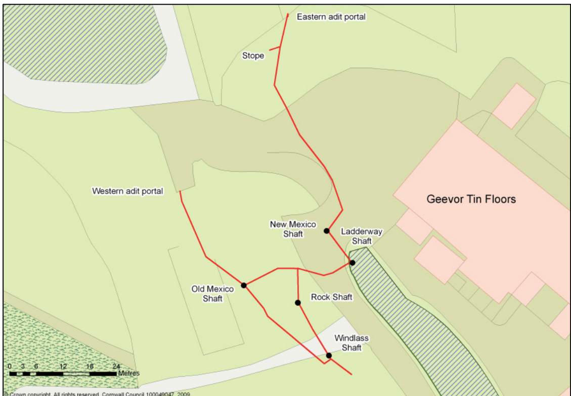
Fig 2. The extent of the project area at Wheal Mexico, showing (in red) the proven sections of the Wheal Mexico shallow adit system. The new extension is the lower section linking Old Mexico Shaft, Windlass Shaft and Rock Shaft.
