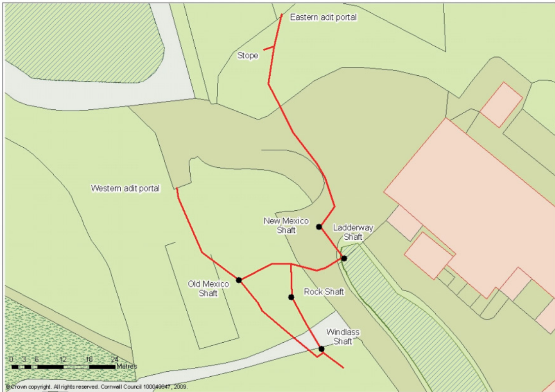
Fig 15. A rectified version of the 2010 Drillserve adit plan. A rectification algorithm incorporated into ArcGis 9.2 was used to geolocate the survey onto the OS Mastermap base. It should be noted that the position of the path from Levant (in grey, bottom of image) does not accurately reflect the position of this feature, which lies a little way to the south.
