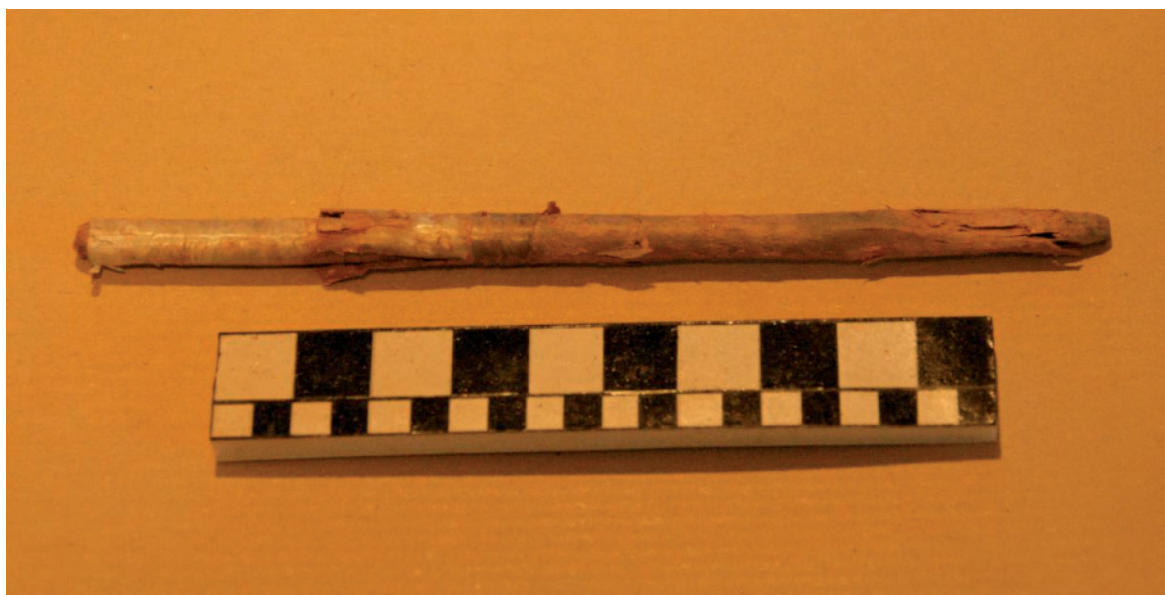
Fig 56. The goose quill fuse found in the western adit backfill. 100mm scale.
