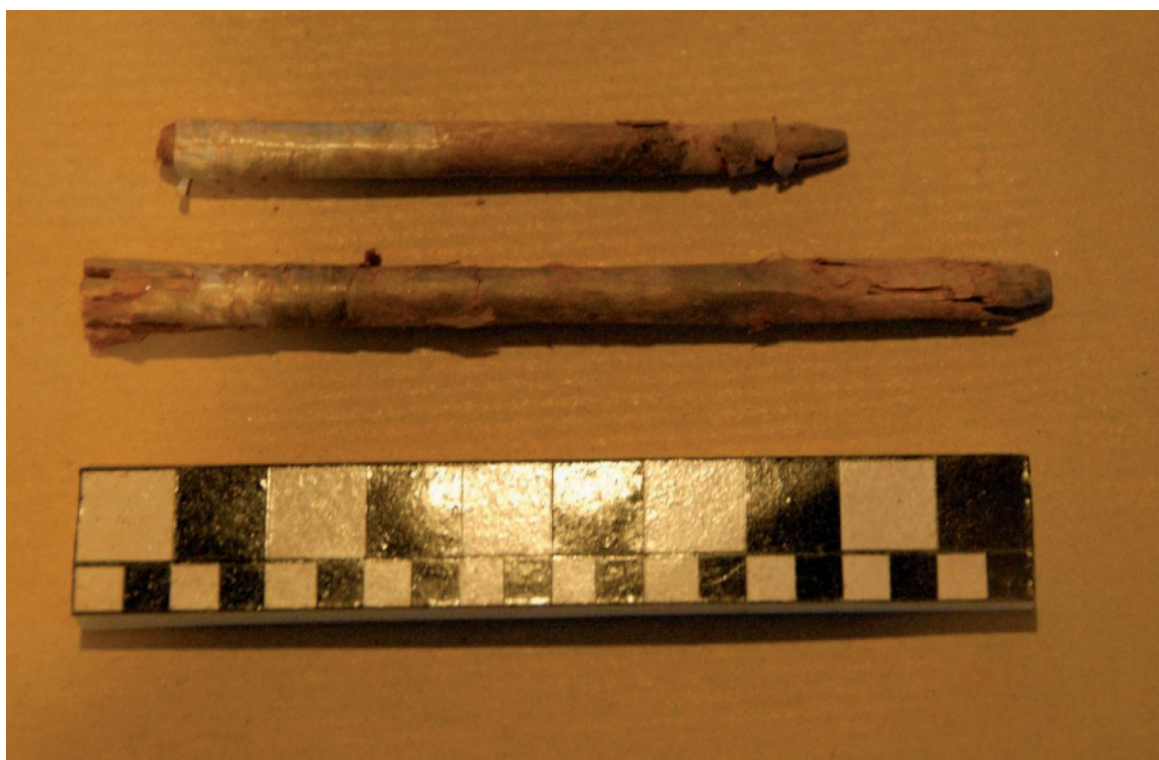
Fig 57. The disassembled goose quill fuse. The material protruding from the left hand end of the upper section is the dried clay which fills it, whilst its reddened section indicates the extent to which it was inserted into the lower piece of quill. 100mm scale.
