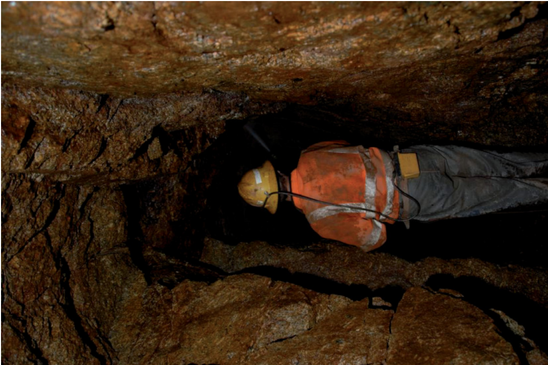
Fig 42. Nick Hall pressure washing slimes from the walls of the western drive.
