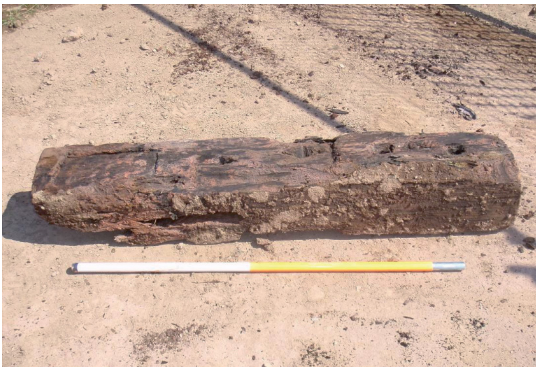
Fig 50. One of the timbers recovered from the eastern stope. Although last used as a prop to support the hanging wall, it had clearly previously been used for other purposes.
