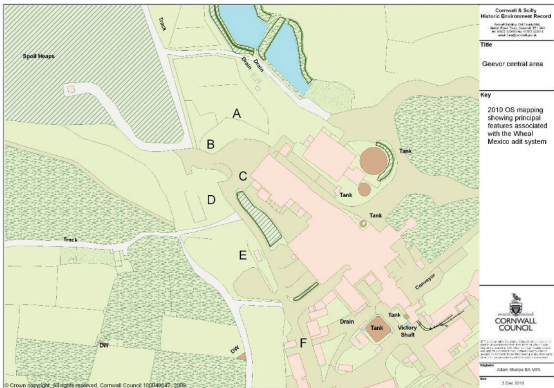
Fig 16. Features associated with the Wheal Mexico adit system. A) Adit entrance, B) Adit exit, C) New Mexico Shaft, D) Sulphide Bay, E) Assay Hut, F) Carpenters' Shop.
