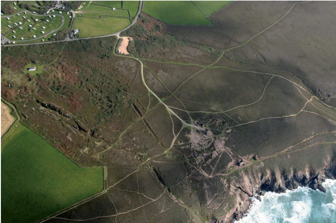
Fig 36. An aerial view of Wheal Coates showing the building complex at the clifftops, the openwork (left), outcrop working pit (left centre), leats (centre) and clay pits (top centre). Also visible is the extensive path network and the considerable erosion around the building complex. HE F68-041.
