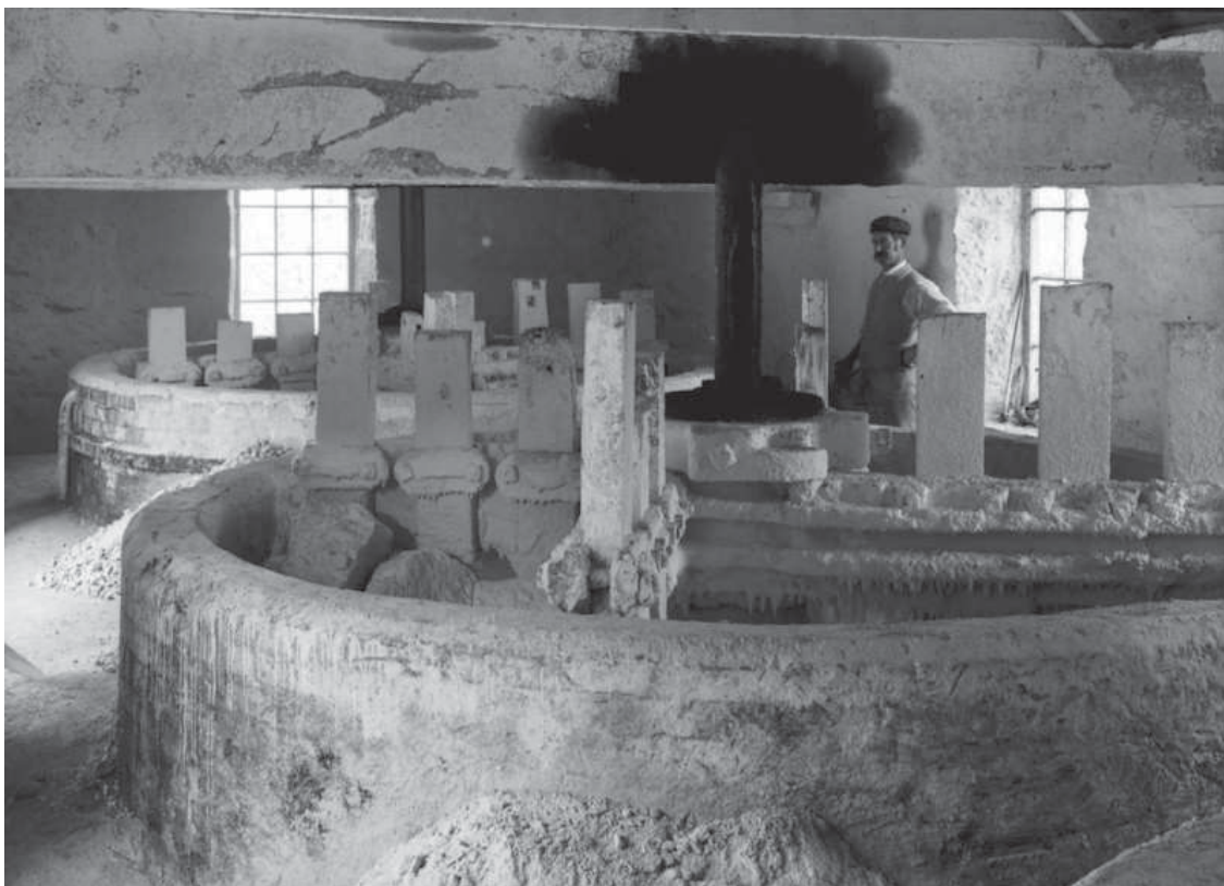
Fig 22. An archive view of the interior of Big Wheel Mill, showing two of its grinding pans. British Geological Survey © NERC. All rights reserved. IPR/121-15CT
