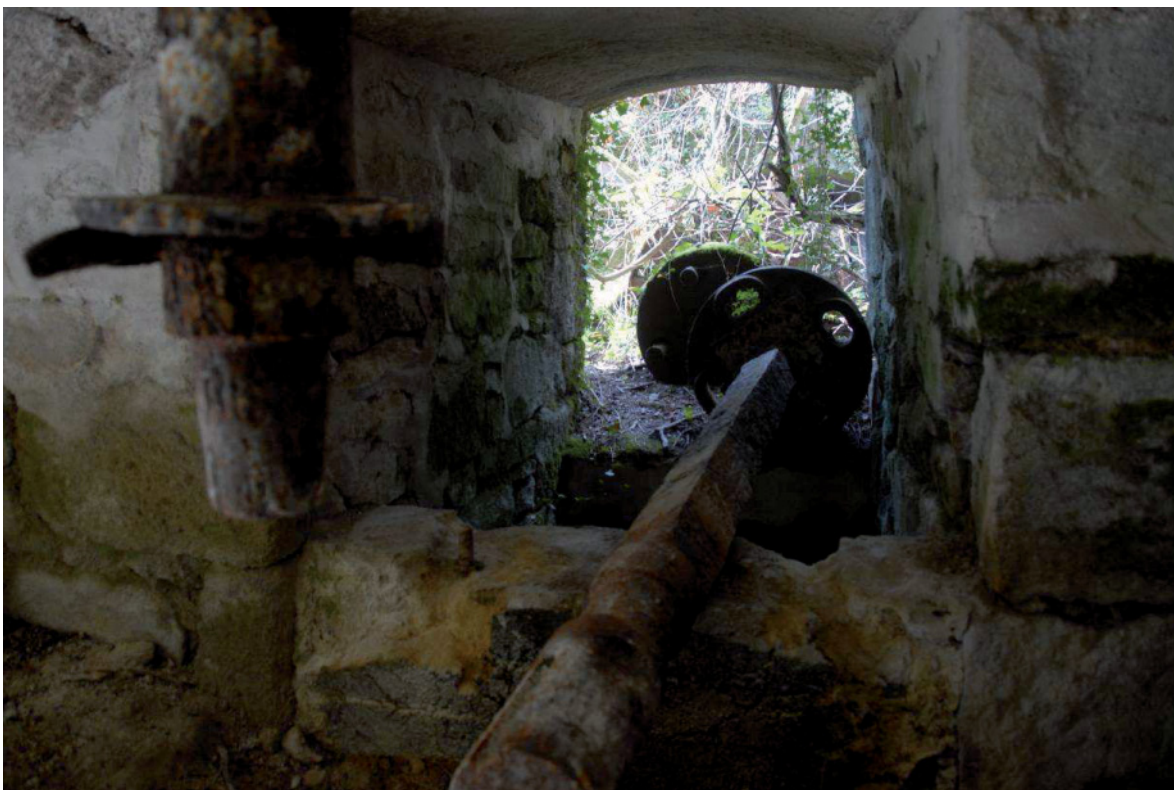
Fig 35. The under-floor axle from the water wheel and one of the vertical axles driving the grinding pans in the southern section of Wheal Arthur china stone mill [10]. HE Digital Image Archive.
