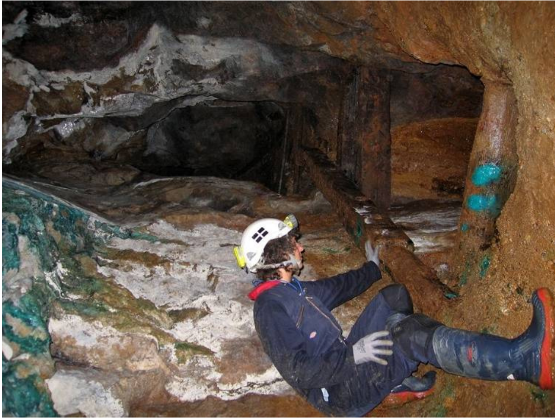
Fig 33. A mine explorer examining the open winze linking the upper and lower adits at Old Engine Shaft. Note the copper staining in the roof of the adit.
