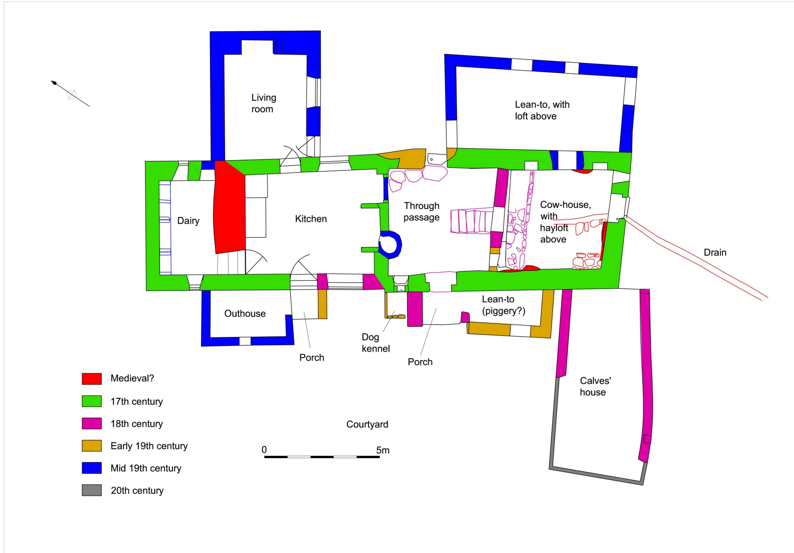
Fig 39 Conjectural phase plan of Codda farmhouse (Based on CAU 1999 survey, with sketch additions).
