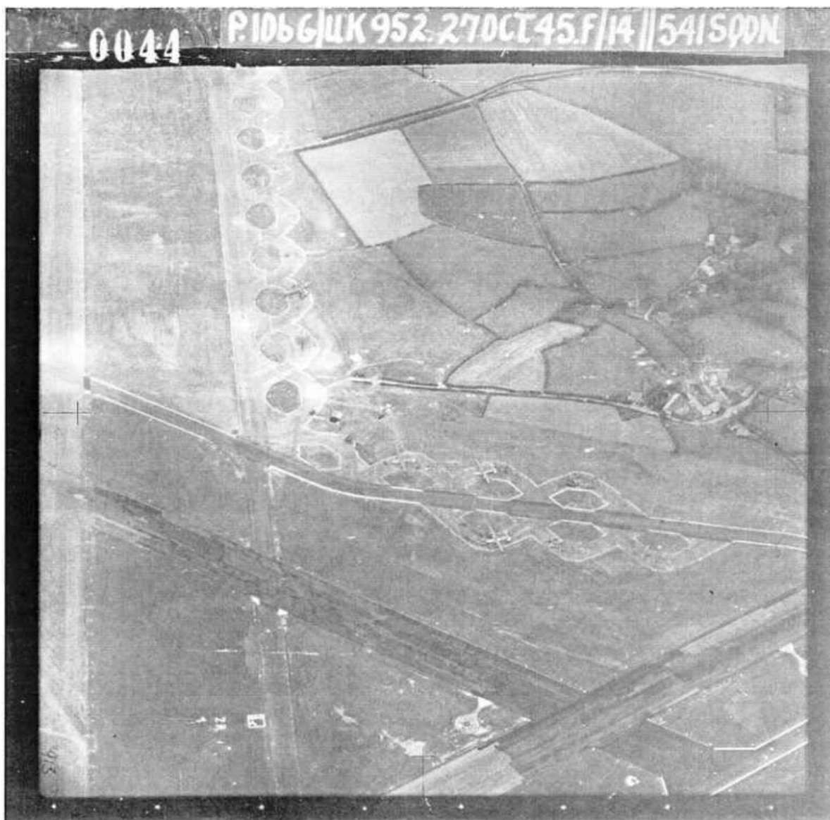
Fig 5 Oblique RAF aerial photograph looking NW across the bottom end of the Northern Loop and up the northern taxiway (in the area of the present terminal complex). To the left is the main runway. Note aircraft on dispersals. (NMR RAF/106G/UK/952/ PSFO 0044 27-OCT-1945). English Heritage (NMR) RAF Photography.
