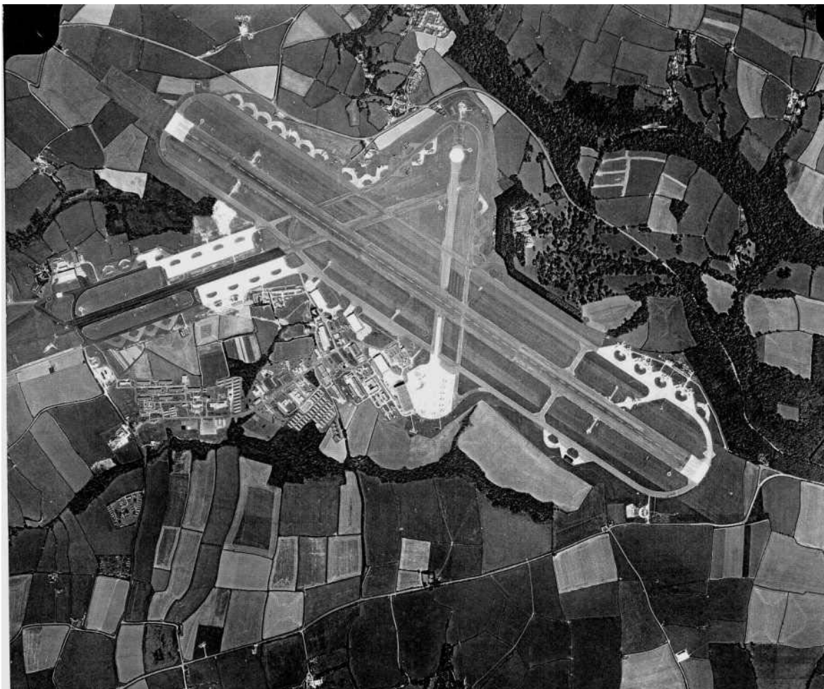
Fig 8 Vertical aerial photograph taken by the National Soil Research Institute in 1971. The arrival of the Nimrod to RAF St Mawgan resulted in the construction of three large apron areas (note the colour of the new concrete), the Nimrod servicing hangar, and the re-arrangement of NE dispersal. Nimrod MR1 aircraft and Canberra aircraft can be seen waiting on the servicing apron and at NE dispersal. (NMR MAL/71131 V 70 5-SEP-1971). English Heritage (NMR) RAF Photography.
