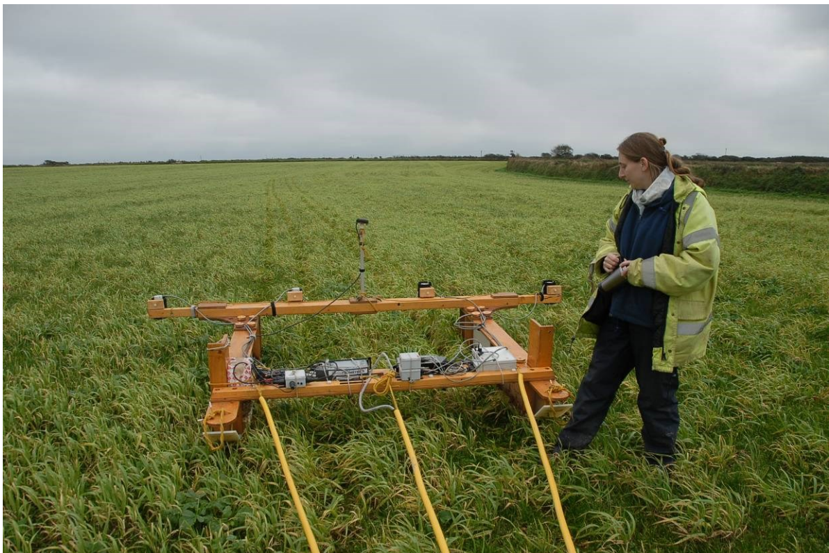
Fig 24. Anne Roseveare of Archaeophysica with the sled-mounted four sensor magnetometer rig. Note the minimal impact its use has had on the young barley crop.
