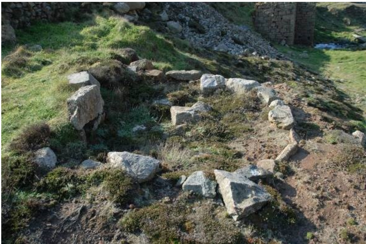
Fig 32. One of the small round buddles to the west of the arsenic calciner where the calcined tin would have been cleaned up at the end of the dressing process.
