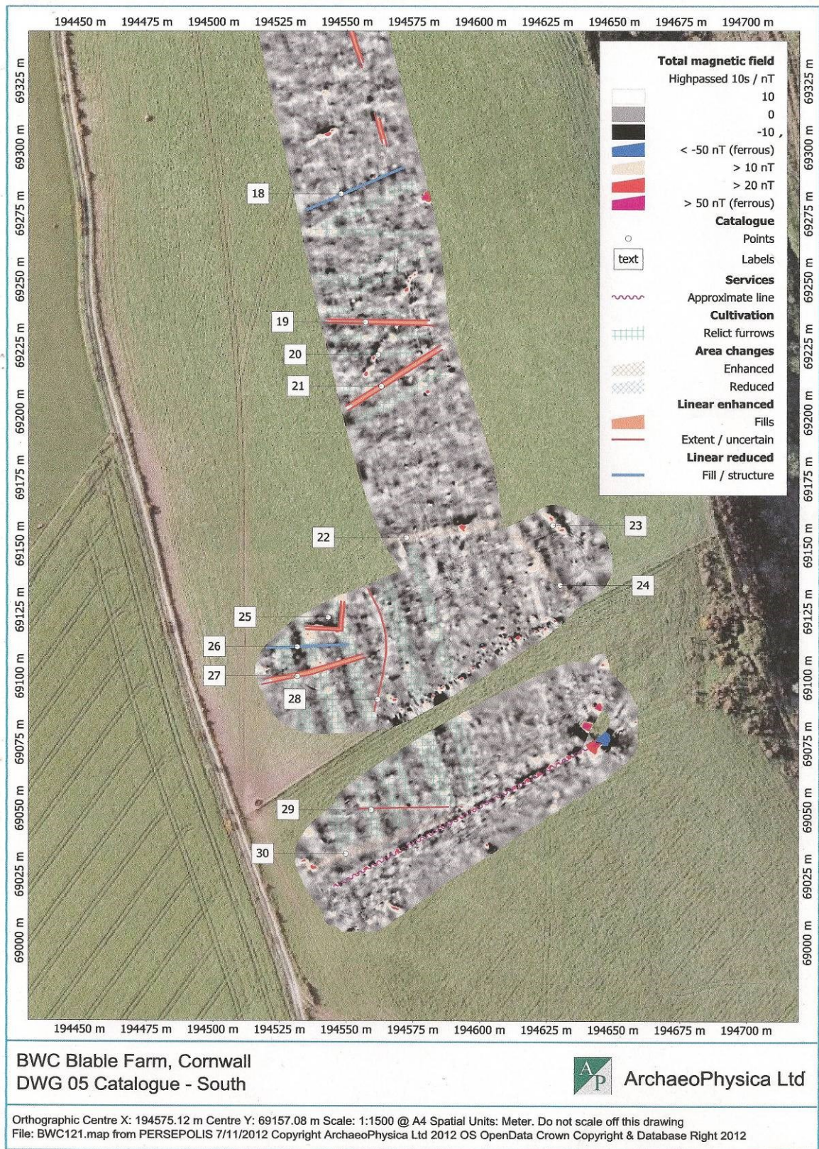
Fig 52. Geophysical survey results from the southern part of the project area. Note the curving feature [28] which may be of early date and the rectangular feature [25] which may be the base of a modern water tank.
