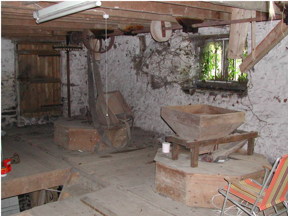
Fig 31 Millstones and machinery (complete with wooden covers and hopper feeds) at Poughill mill, Stratton
