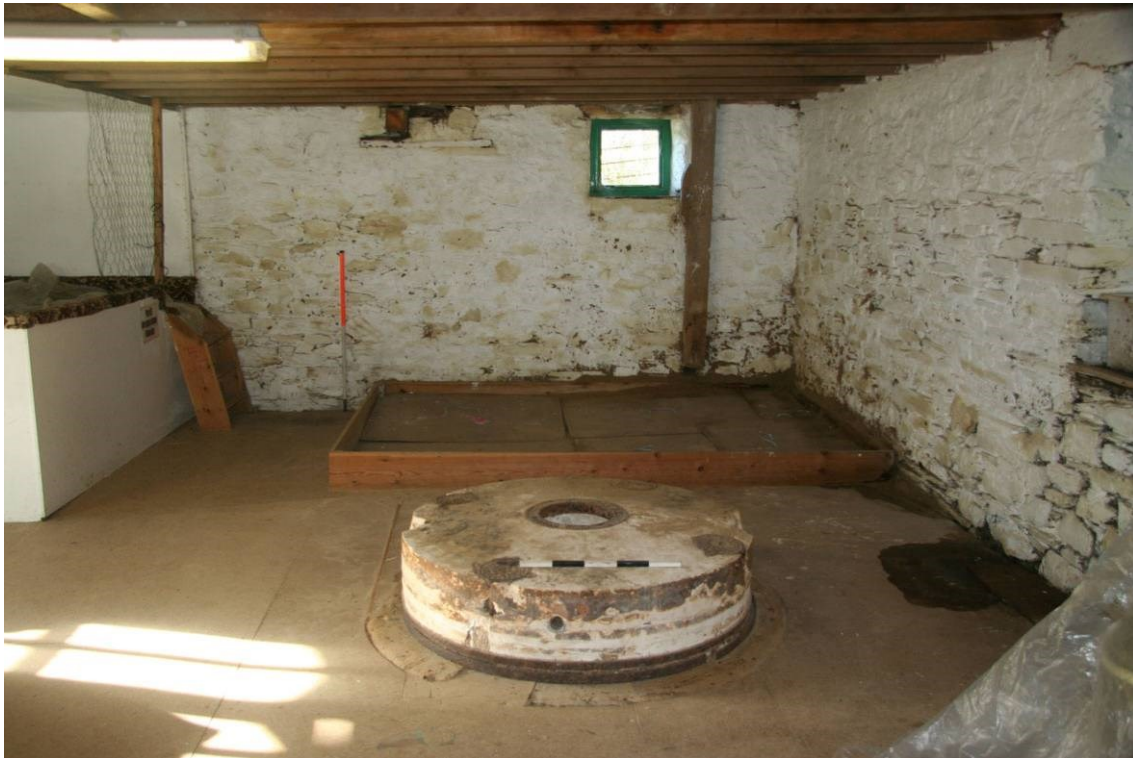
Fig 29 The single surviving set of millstones on the first floor, now without wooden covers (compare with a more complete example in Fig 31)
