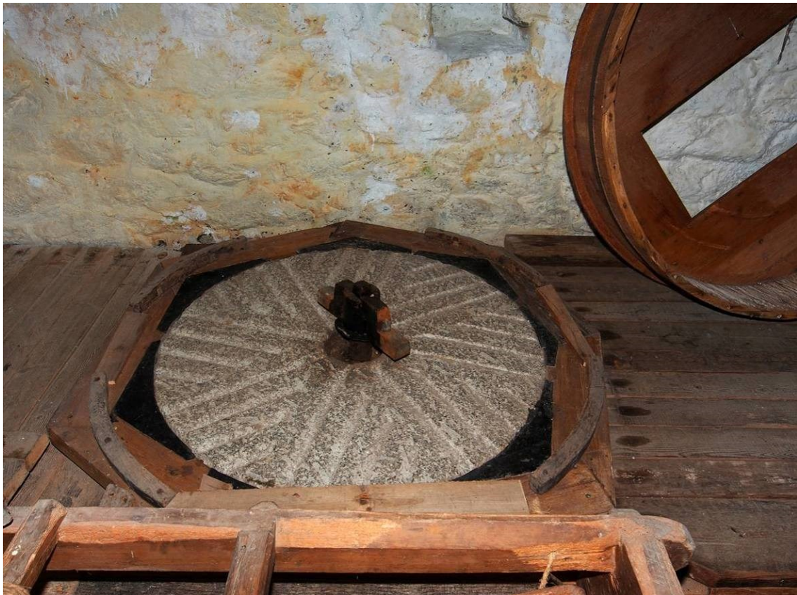
Plate 36 The western mill bedstone in situ
