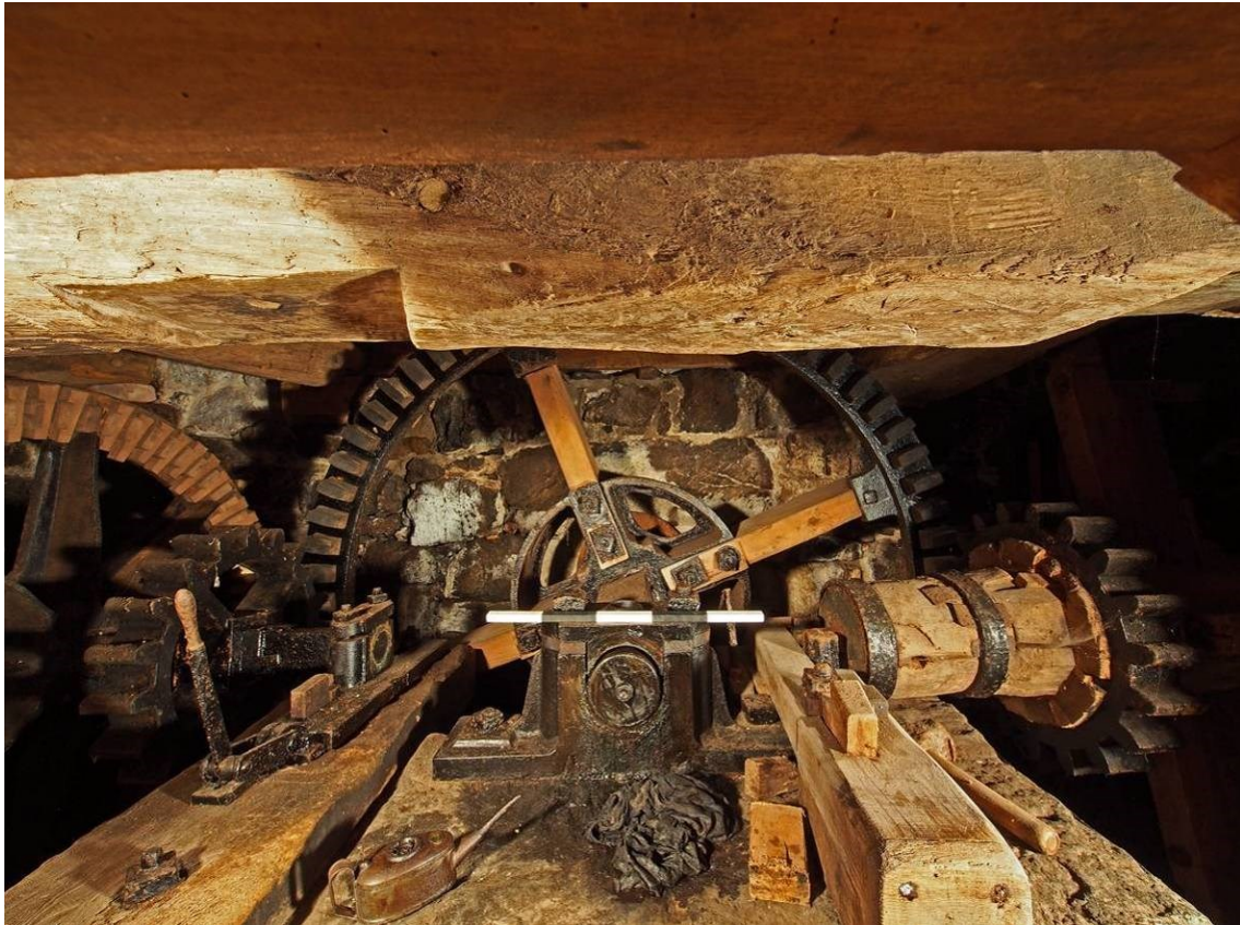
Plate 27 Pit wheel (behind, centre) sharing axle with waterwheel, driving horizontal countershafts to secondary gearing onto stone nuts driving millstones
