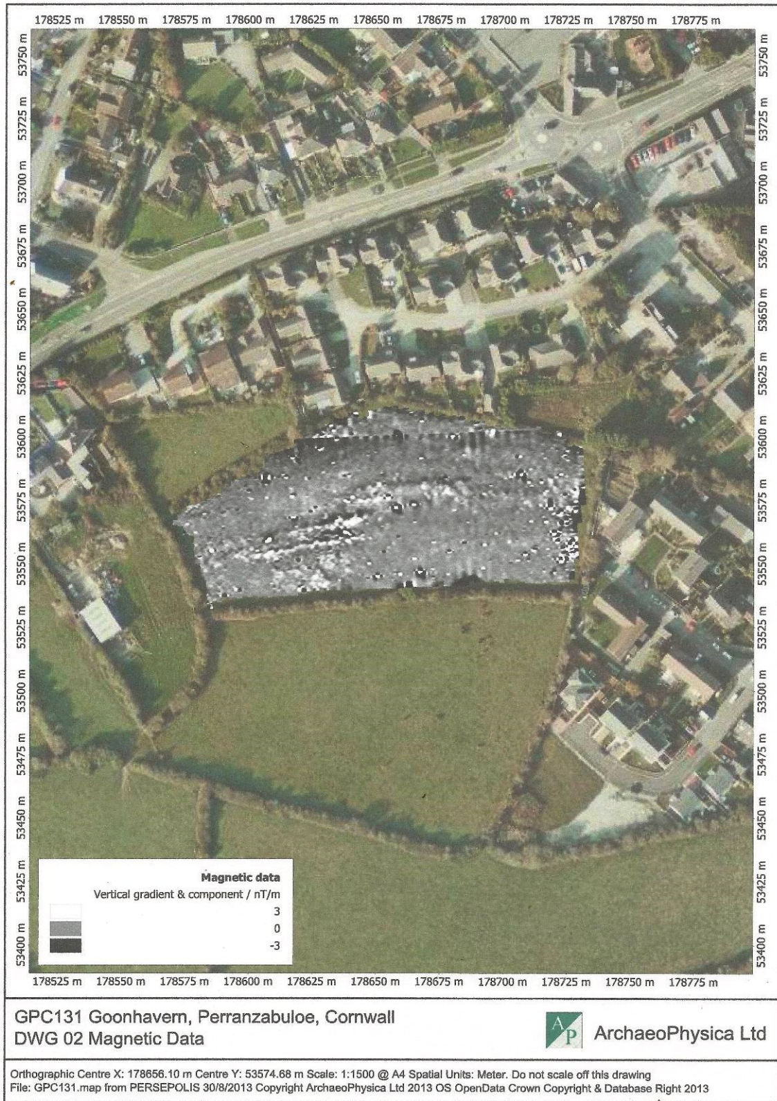
Fig 19. The geophysics data plot for the Goonhavern site. Several linear features are evident in the data, as well as the notable cluster of dipolar responses at the eastern end of the site.
