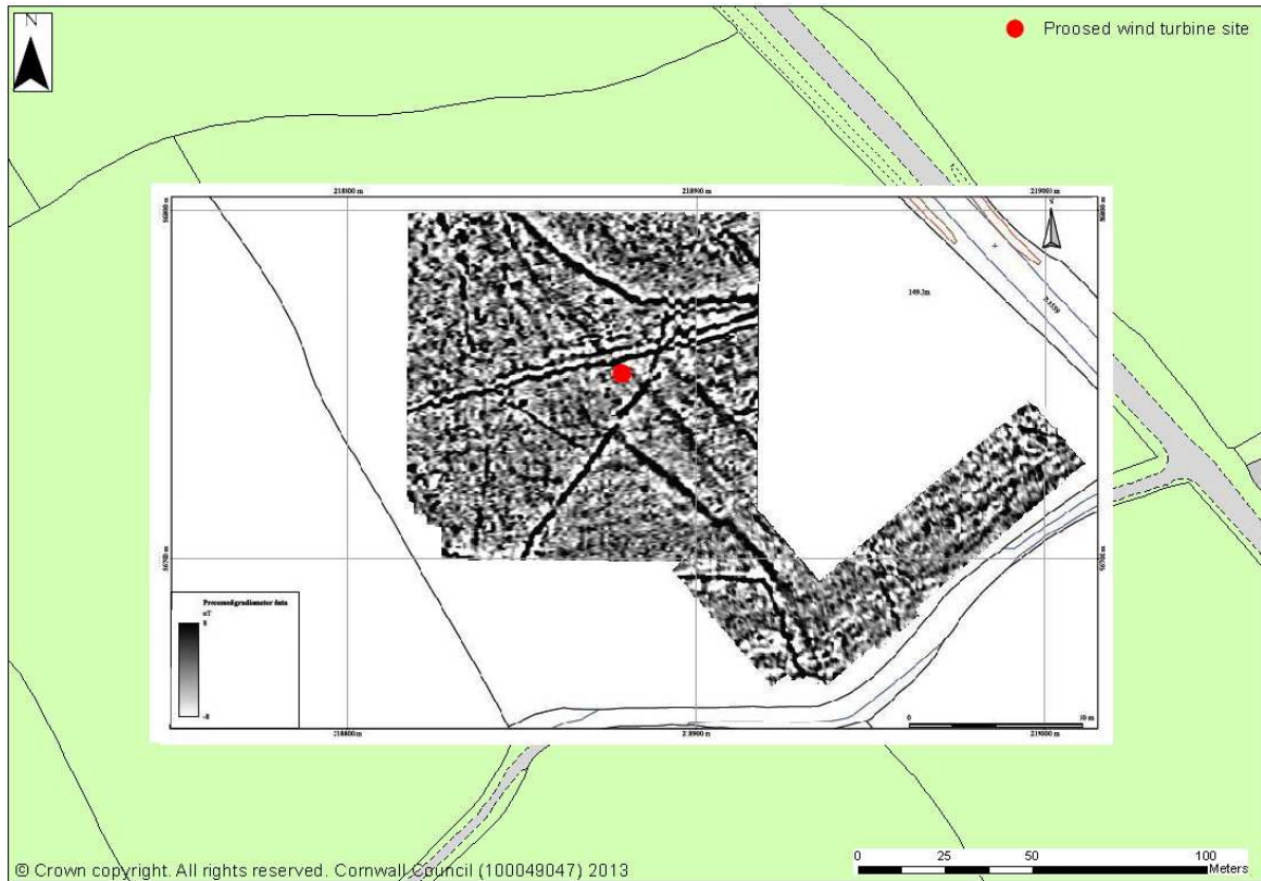
Fig 49 Results of the geophysical survey at Tresawson by Substrata, georeferenced onto the OS Mastermap and showing the proposed wind turbine site.
