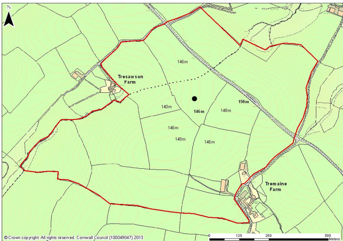
Fig 12 OS contour data for the area immediately surrounding the proposed wind turbine shows its site located on a north west facing slope between two small hill tops
