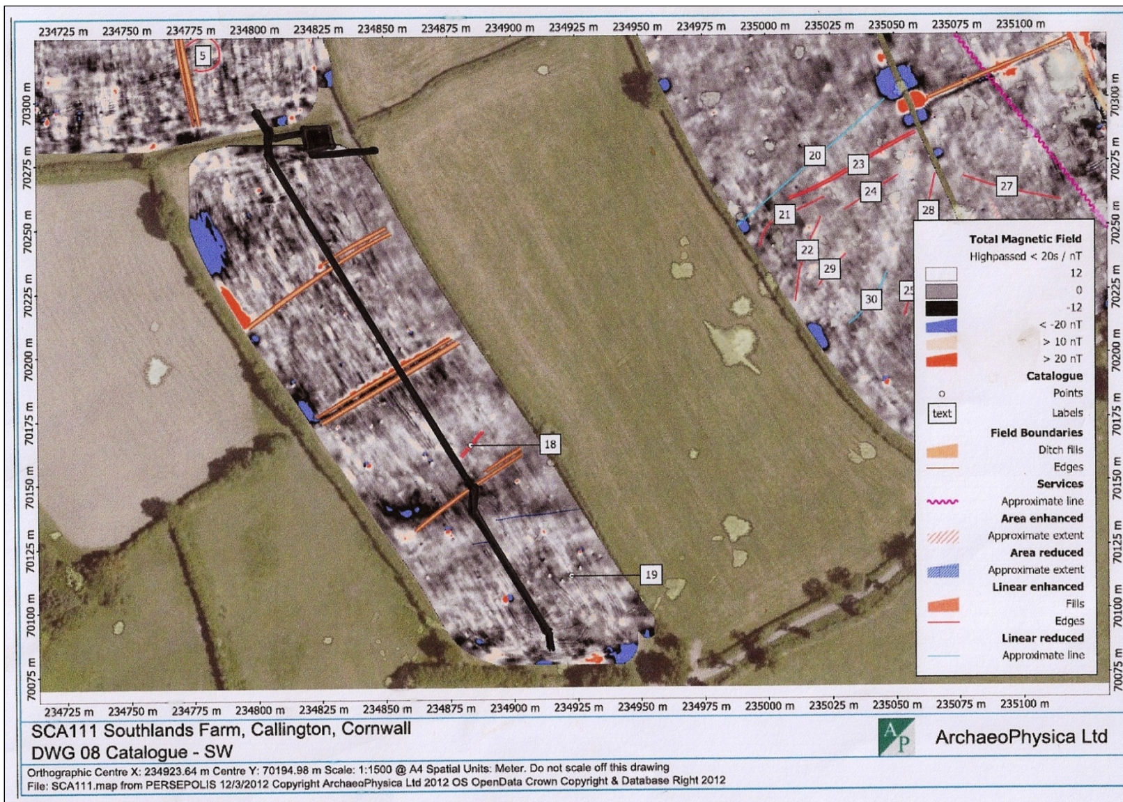
Figure 6 Geophysics data for Field C (see Figure 2 for site locations), with main cable and transformer duct trenches shown in black intersecting possible archaeological features
