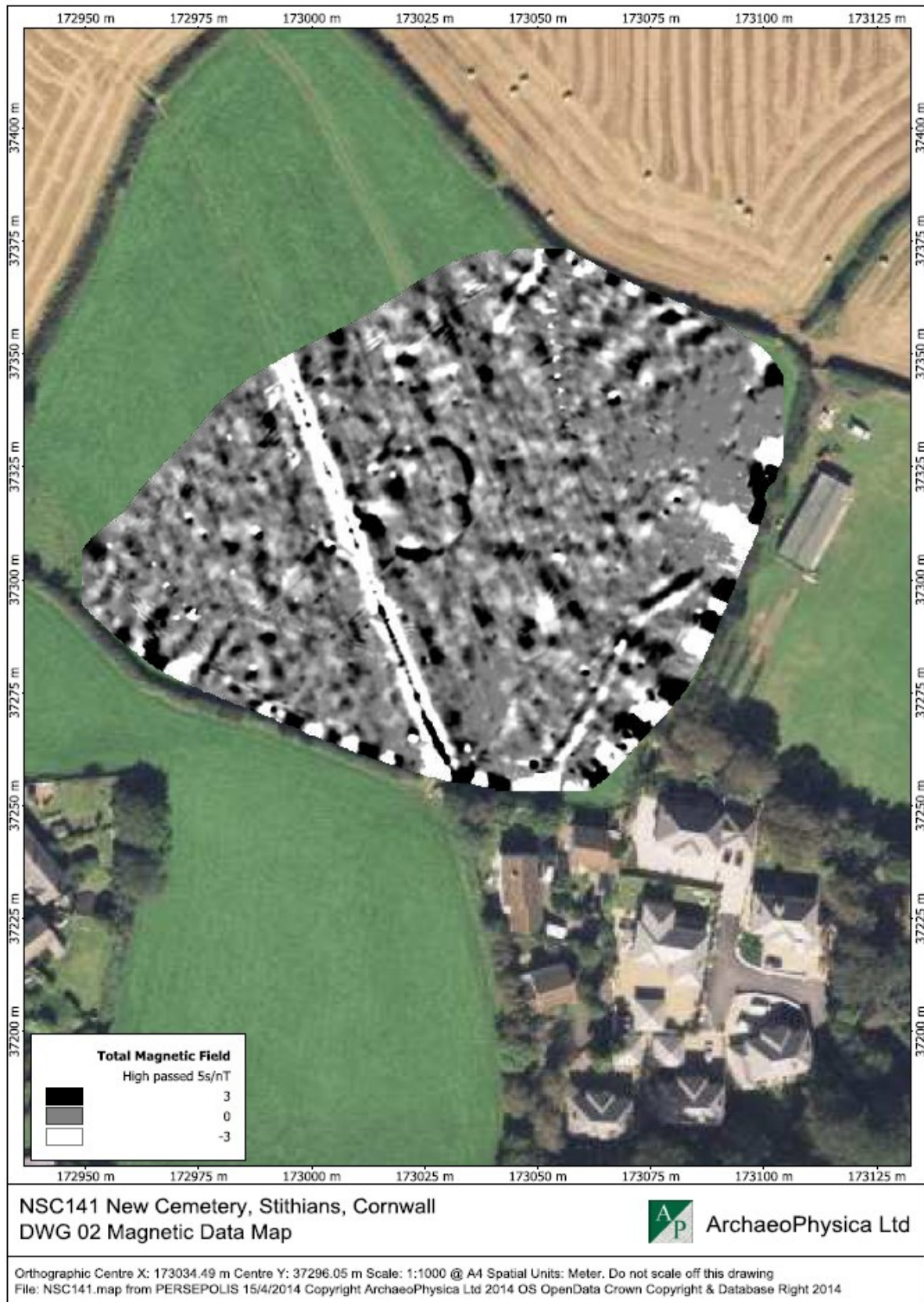
Fig 7 The geophysics data plot for the Stithians cemetery site. Several linear features are evident, as well as a cluster of discontinuous arcs making up a sub-circular feature. NB. The area over which the geophysical survey was conducted extended over the proposed cemetery site but also covered an additional area to the west.
