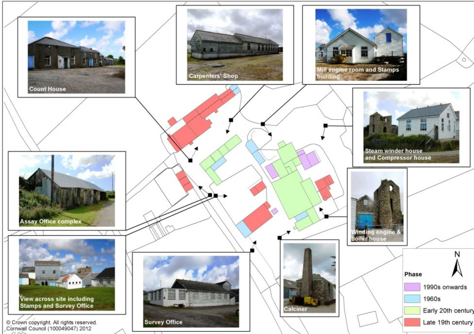
Figure 3 A plan showing existing views of King Edward Mine transposed onto a phase map of site development. Only the Assay, Boiler house, and Mill buildings are relevant to this report
