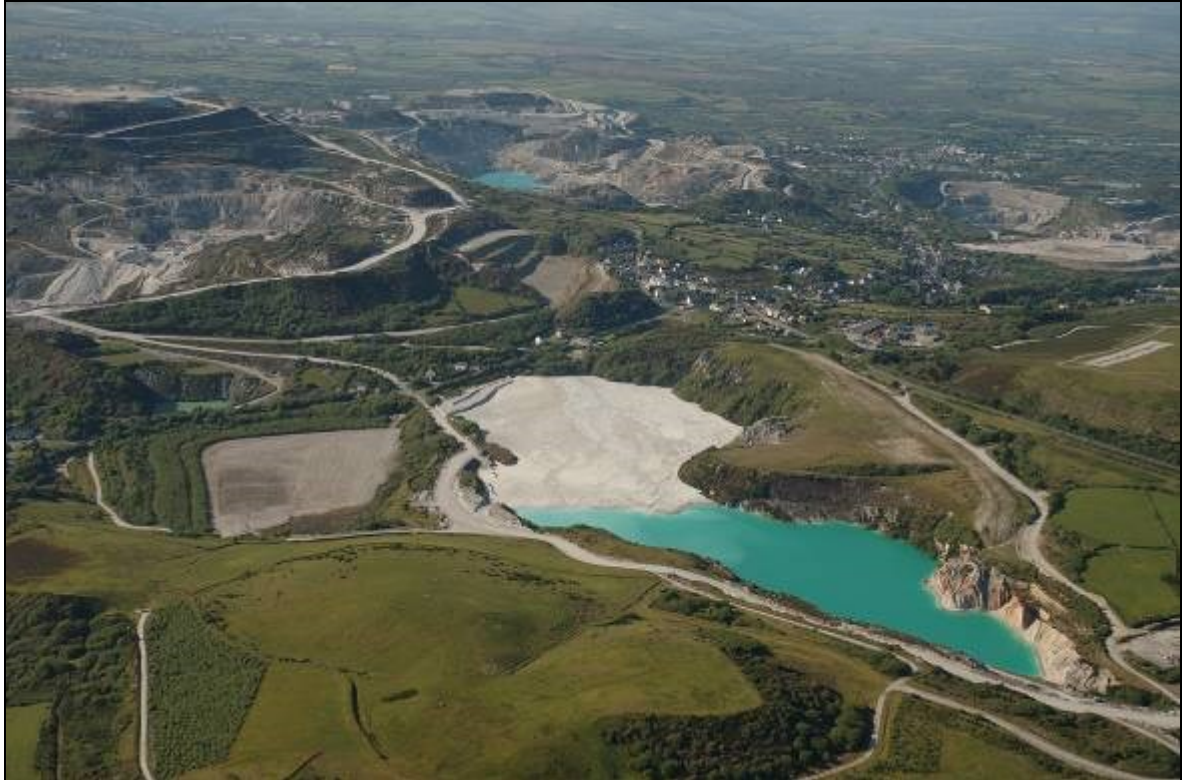
Fig 111 The dynamic character of the clay industry landscape is evident in the backfilling with waste of the former Lower Ninestones (left) and Penhale pits, the re-profiling and re-vegetation of former tips in the foreground and active working at Gunheath and other sites in the distance. (Photograph: Historic Environment, Cornwall Council: F67-029; 8 June 2005.)
