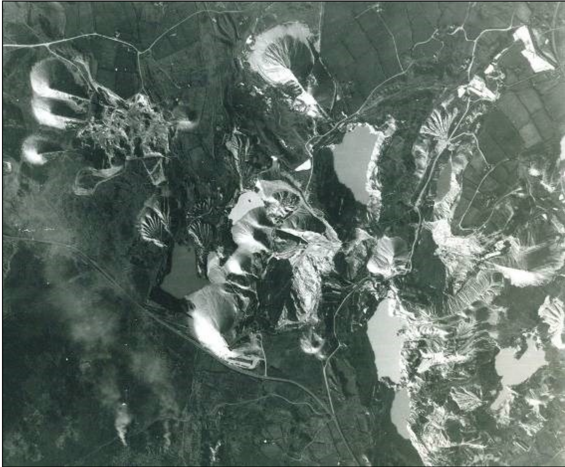
Figure 94 A vertical air photograph of clay operations on the northern flank of the Hensbarrow Downs in April 1947; north to the top. At centre left the flooded pits of the former Great Wheel Prosper and West Goonbarrow clay works, both marked out as an earlier generation of working by well-defined fans of finger dumps, are in the process of being backfilled with waste from the operational North Goonbarrow pit to the south east. Much of the southern end of Great Wheel Prosper pit was infilled, although part survives; West Goonbarrow pit appears to have been completely backfilled. The workings and enclosed land across almost the whole of the right hand side of the image have subsequently been absorbed by the modern Goonbarrow pit and associated infrastructure. (Photograph: RAF CPE/UK 1999/B32/4135; 13 April 1947. Print held by Cornwall Council Technical Services.)
