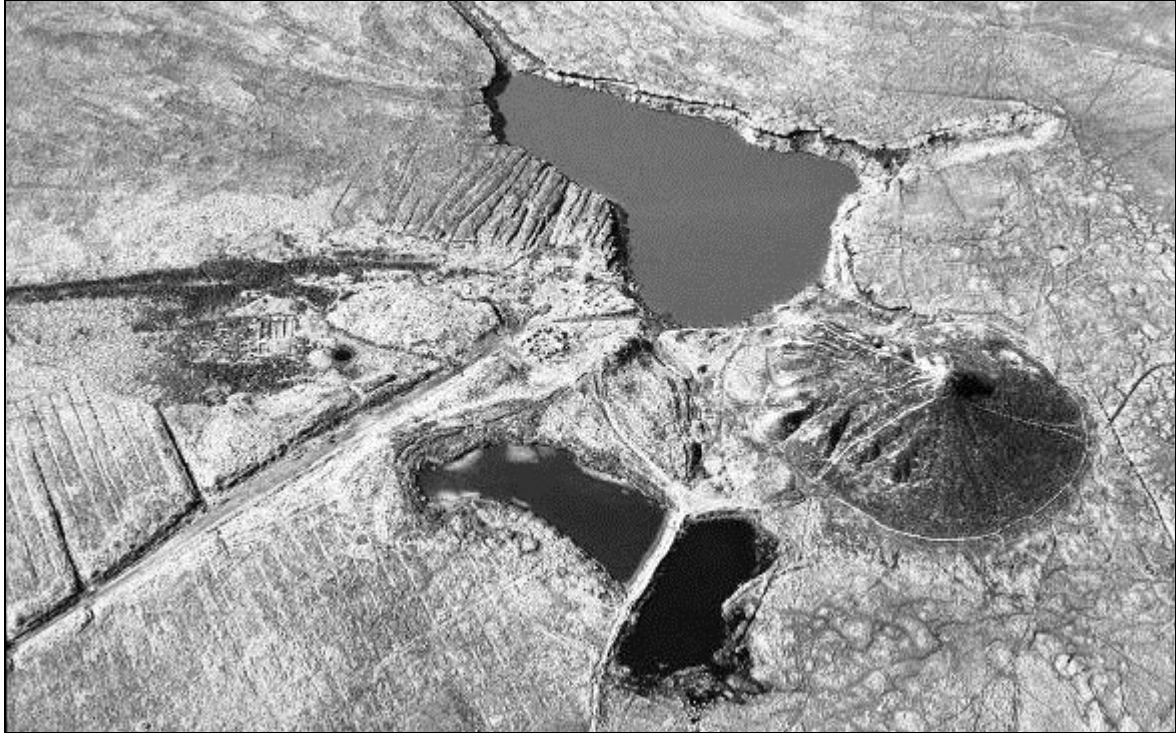
Figure 29 The remote Redlake china-clay works on southern Dartmoor opened in 1913 with total initial investment exceeding £100,000. The site was served by a 13 km tramway and liquid clay produced there was shipped by gravity to settling tanks and kilns off the moor at Cantrell, on the Great Western Railway main line. The operation closed in 1932. (Photograph F M Griffith, Devon County Council, 16 February 1988.)
