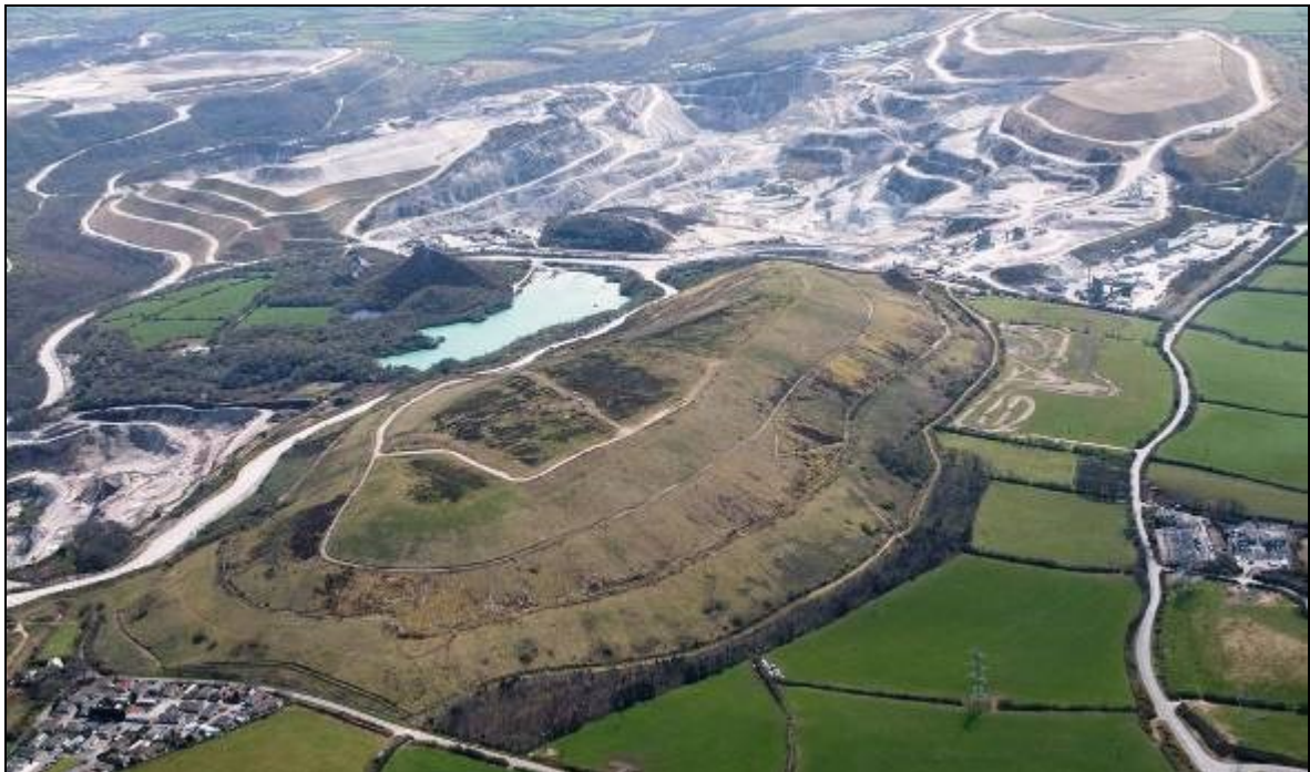
Figure 74 A re-profiled late twentieth-century tip on the former Burthy Downs, south of Fraddon on the western edge of the St Austell china-clay district. The rounded, smoothed and symmetrical form of the tip, which is visible over a wide area to the west, partly conceals its industrial origins but is uncharacteristic of the natural landforms of the St Austell granite. (Photograph: Historic Environment, Cornwall Council: F82-003; 16 April 2008.)
