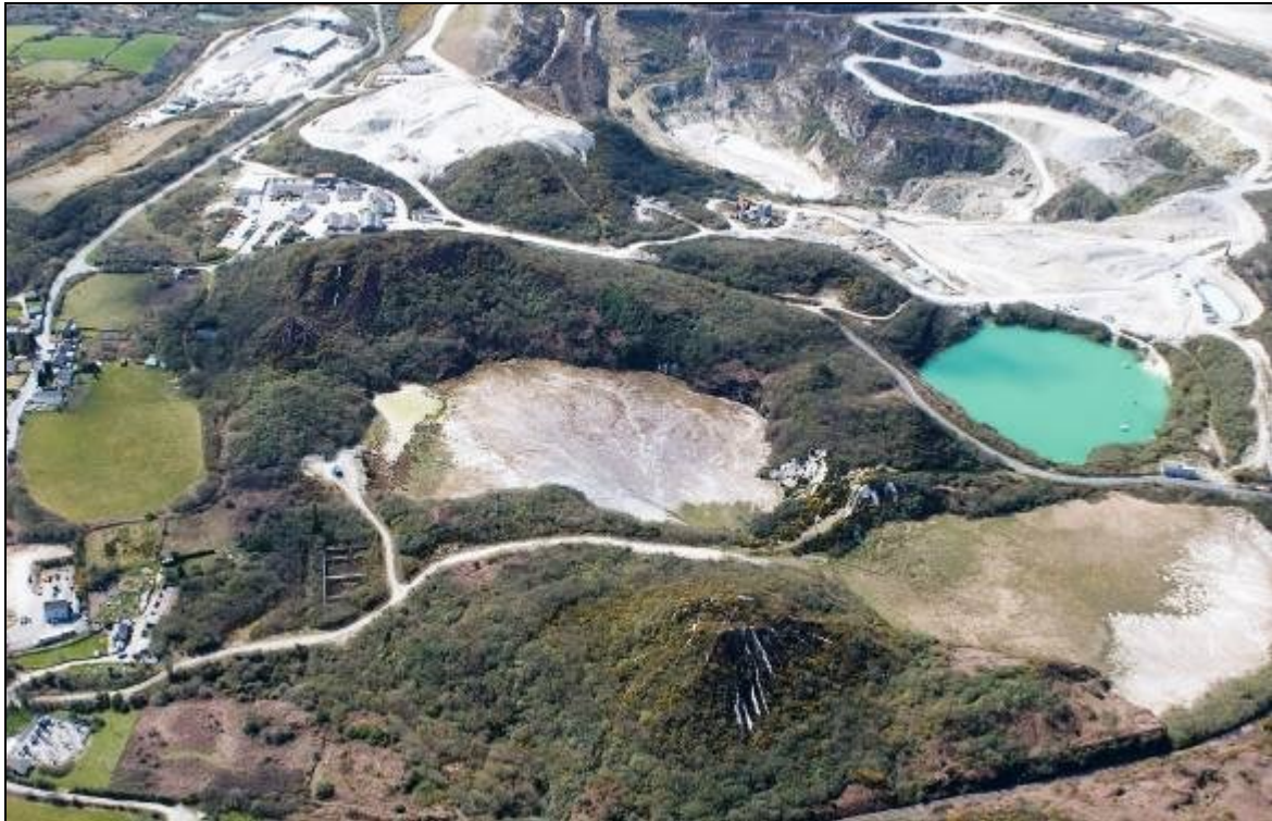
Figure 95 Two of three former pits at Bloomdale, Goonamarris, in the St Austell clay area, have been backfilled with mica waste. (Photograph: Historic Environment, Cornwall Council: F82-009; 16 April 2008.)
