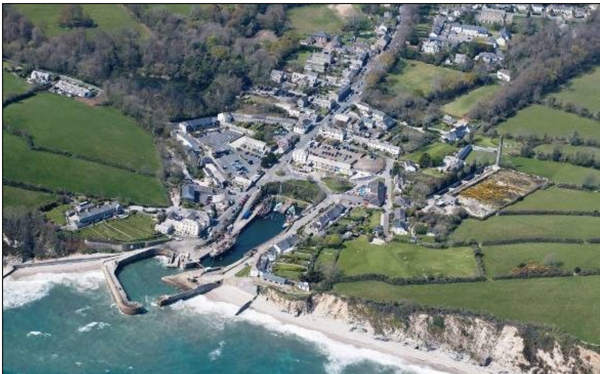
Figure 13 The historic port of Charlestown, looking north west. Constructed during the 1790s, it was important in exporting both china clay and china stone from the early period of the industry. To the right are the remains of a large pan kiln complex built in 1906-7 for the Lovering company and used to refine clay brought by pipeline from Carclaze. (Photograph: Historic Environment, Cornwall Council: F82-127; 16 April 2008.)
