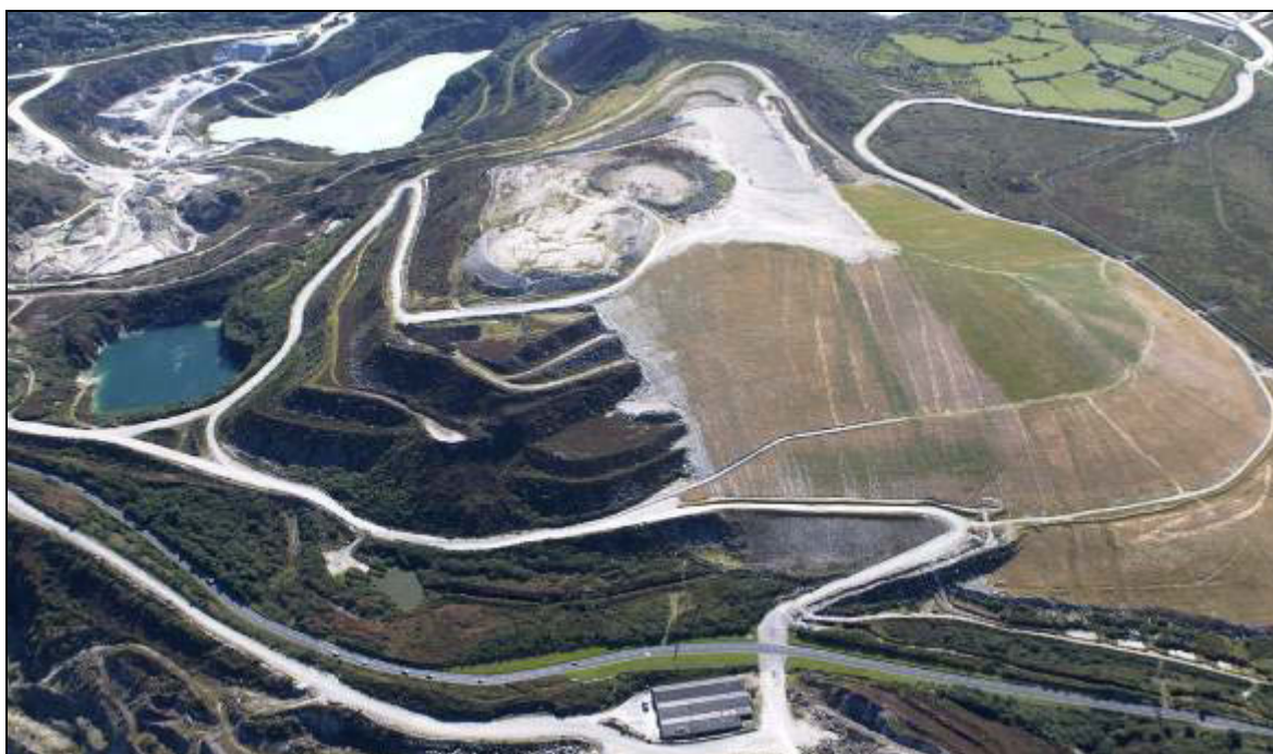
Figure 73 Re-profiling and re-vegetation of modern stepped china-clay waste tips in progress on Hensbarrow Downs in 2009. The characteristic form of the tips created by the modern industry is almost entirely obliterated, leaving a smoothed and rounded landform which shows little of the topographical characteristics of south-western granite uplands. The Bronze Age Hensbarrow (top right), formerly the third highest point in Cornwall and a prominent landmark in the region, is now overtopped and dominated by the tip (cf Fig 47). (Photograph: Historic Environment, Cornwall Council: F95-025; 10 September 2009.)
