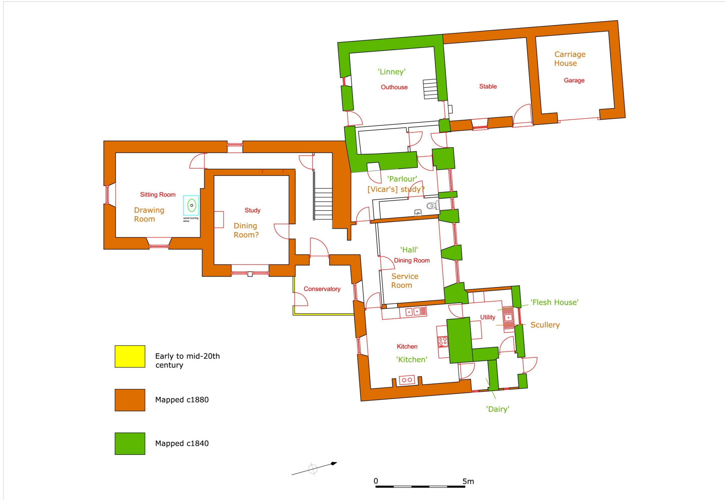
Fig 60 Ground floor plan, showing main phases of development of surviving fabric, with historic room names quoted from terriers or suggested by the assessment
