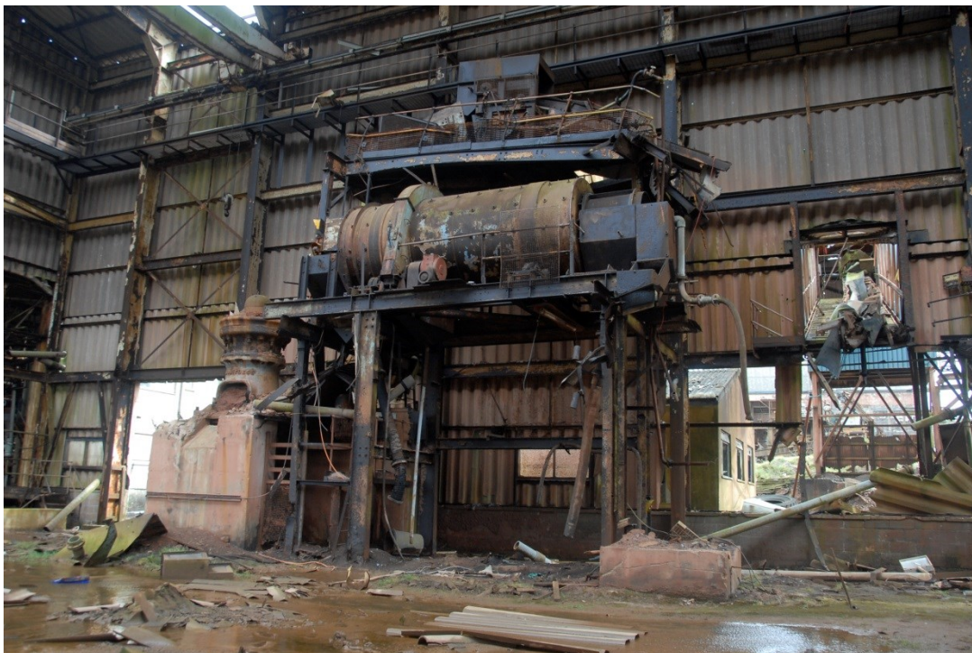
Fig 10. The large ball mill in situ within the primary crusher building.
