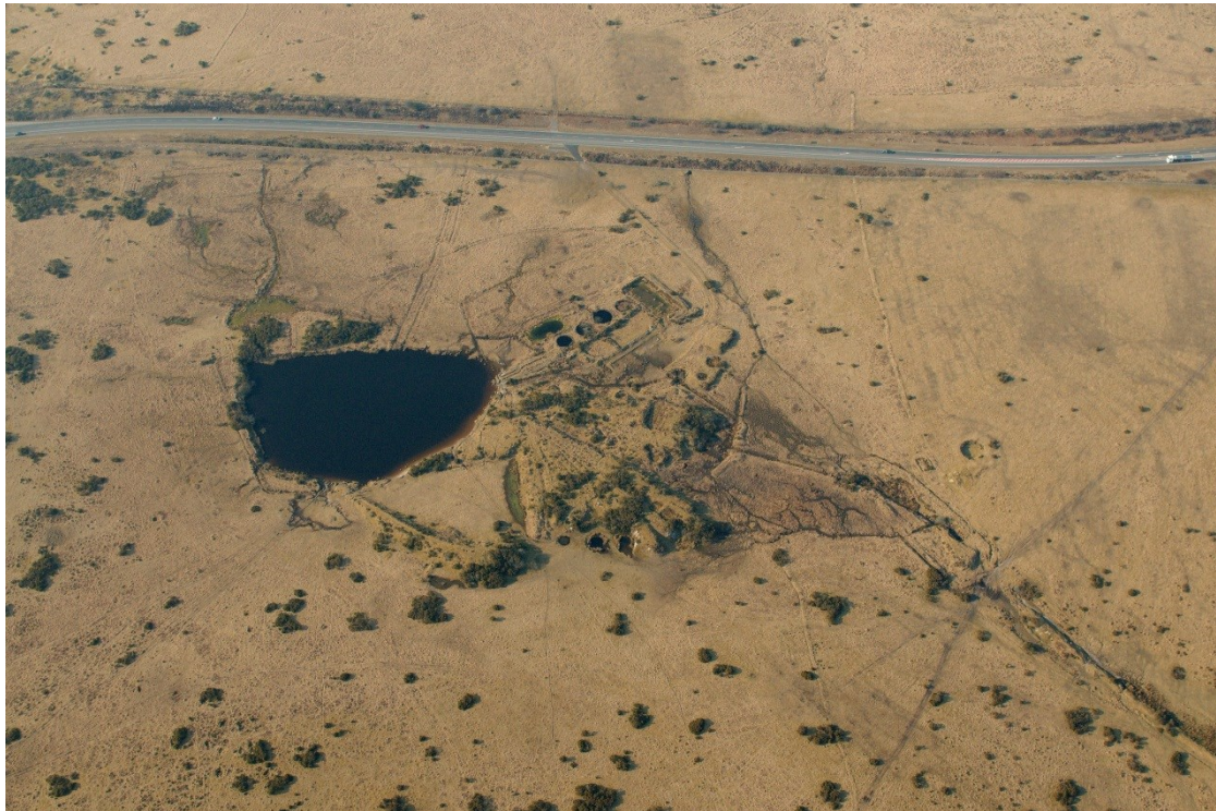
Fig 47. The Burnt Heath china clay works near Temple was small-scale and was only worked for a short period. Its site preserves some now-rare features, including air dries where the finished clay was dried in the open air.
