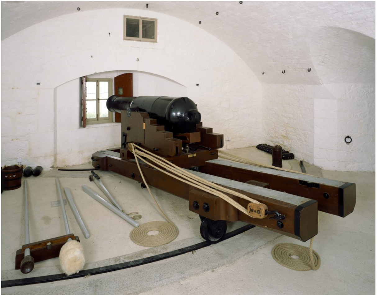
Fig 34 The 19 th century 64pdr RML on its reconstructed traversing slide carriage in the battery casemate.
