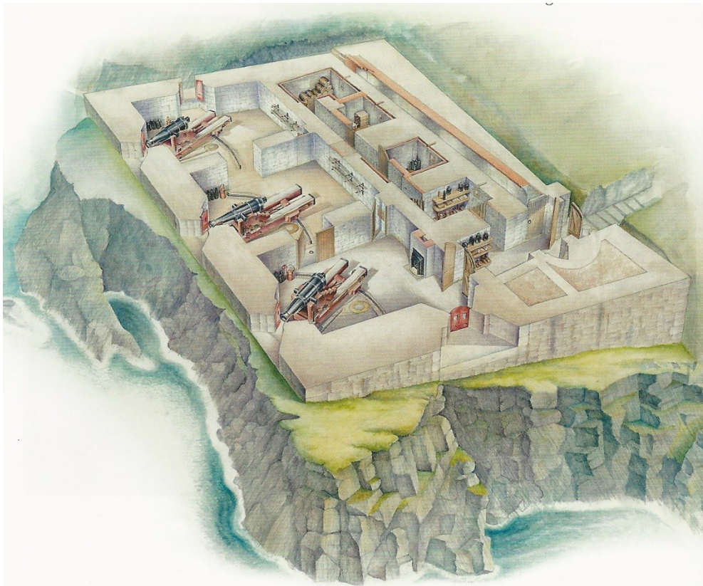
Fig 23. A cutaway drawing of the lower floor of the mid-19 th century gun battery, incorporating its modified magazine area.
