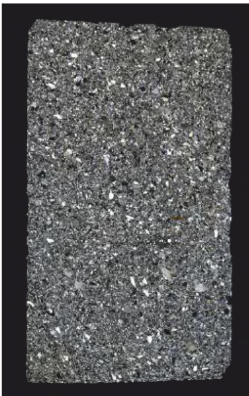
Figure 19. Micro-photograph of thin section through Group XIX greywacke potential axe S101 CO479 (Photograph: Jens Andersen).
