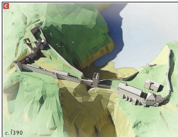
Figs 33 A-D. The development sequence for the Mainland and Island wards during the period from 1260 to 1540 proposed in the current English Heritage guidebook to Tintagel Castle. A – the initial appearance of the castle when constructed. B – parts of the Great Hall and the western wall of the Mainland wards had collapsed into the sea through cliff erosion. C – A new western wall had been constructed for the Mainland wards and lodgings had been built on the site of the Great Hall. D – The drawbridge had collapsed into the sea and the Island ward lodgings had been reduced in size.
