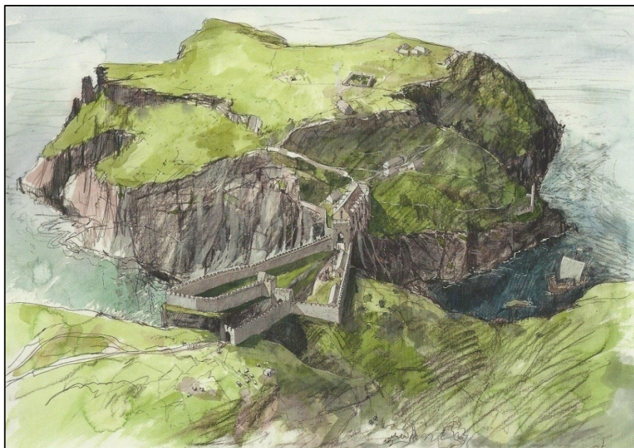
Fig 32. A companion reconstruction showing Tintagel during the 13 th to 14 th centuries, again commissioned from Liam Wales by English Heritage. This model again assumes a narrow, almost completely level upper surface to the isthmus and a drawbridge near the Great Hall.
