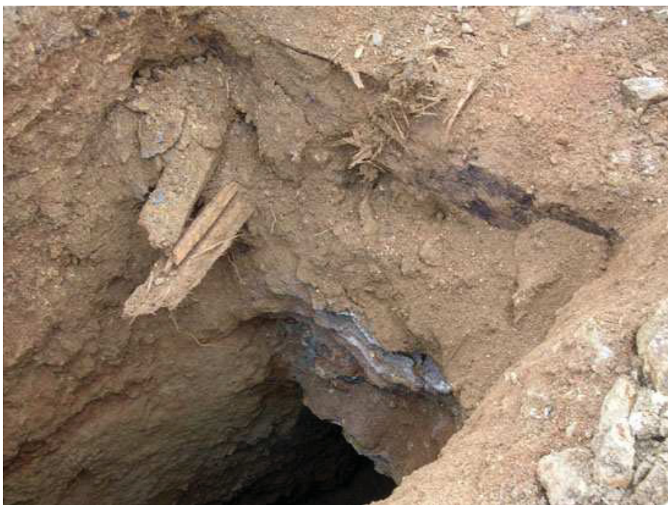
Fig 6: Concrete footings 1.0m below the current ground surface were observed within test pit 22.
