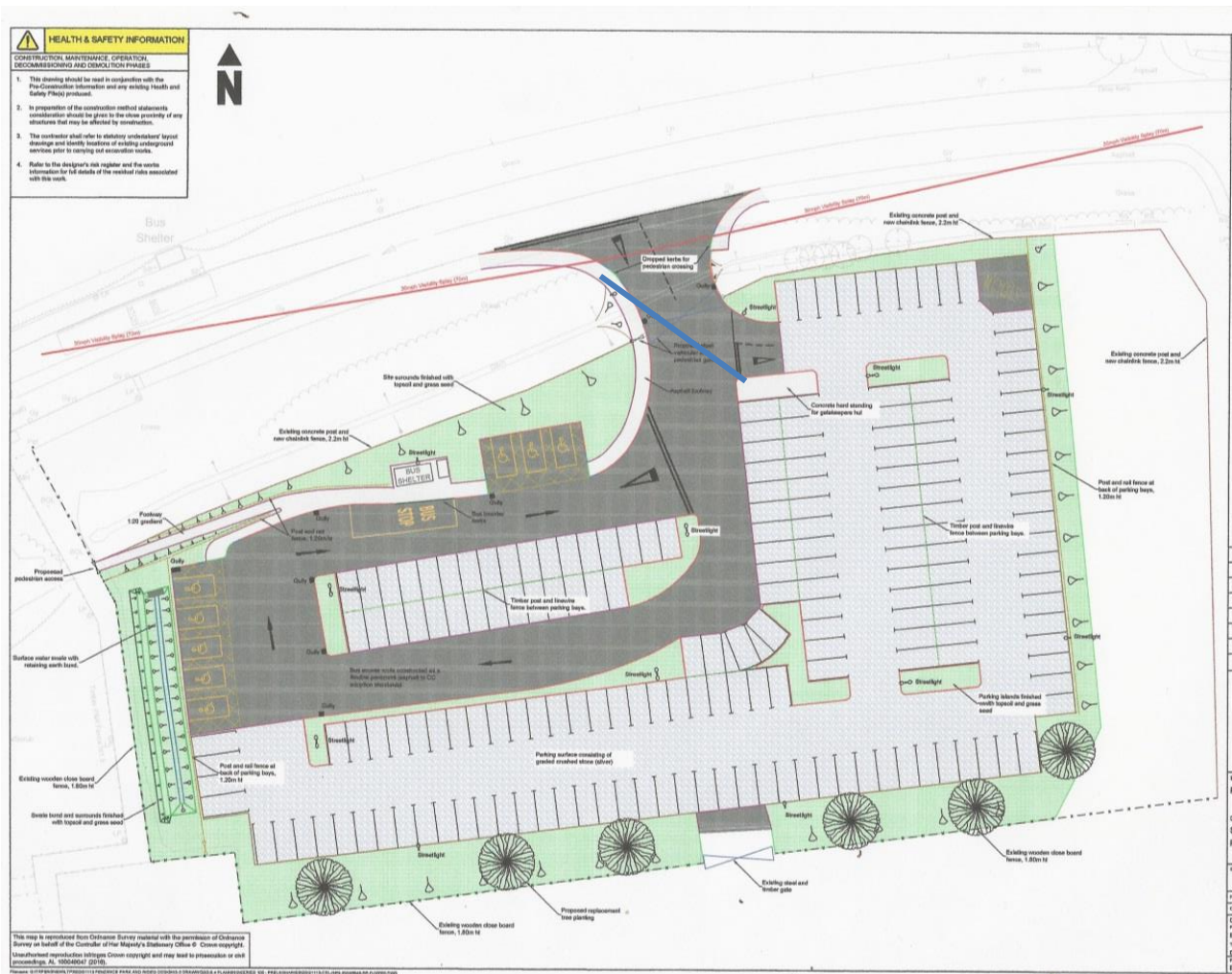
Fig 3. The proposed layout for the Penzance Park and Ride facility. The blue line indicates the approximate line of the new sewer trench.
