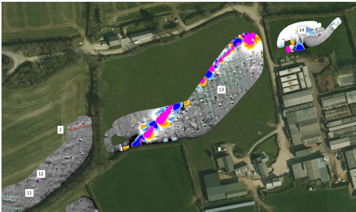
Fig 13. Geophysical results from the central area. [13] indicates an area of cultivation activity. The brighter colours derive from a buried metal pipe or similar.
