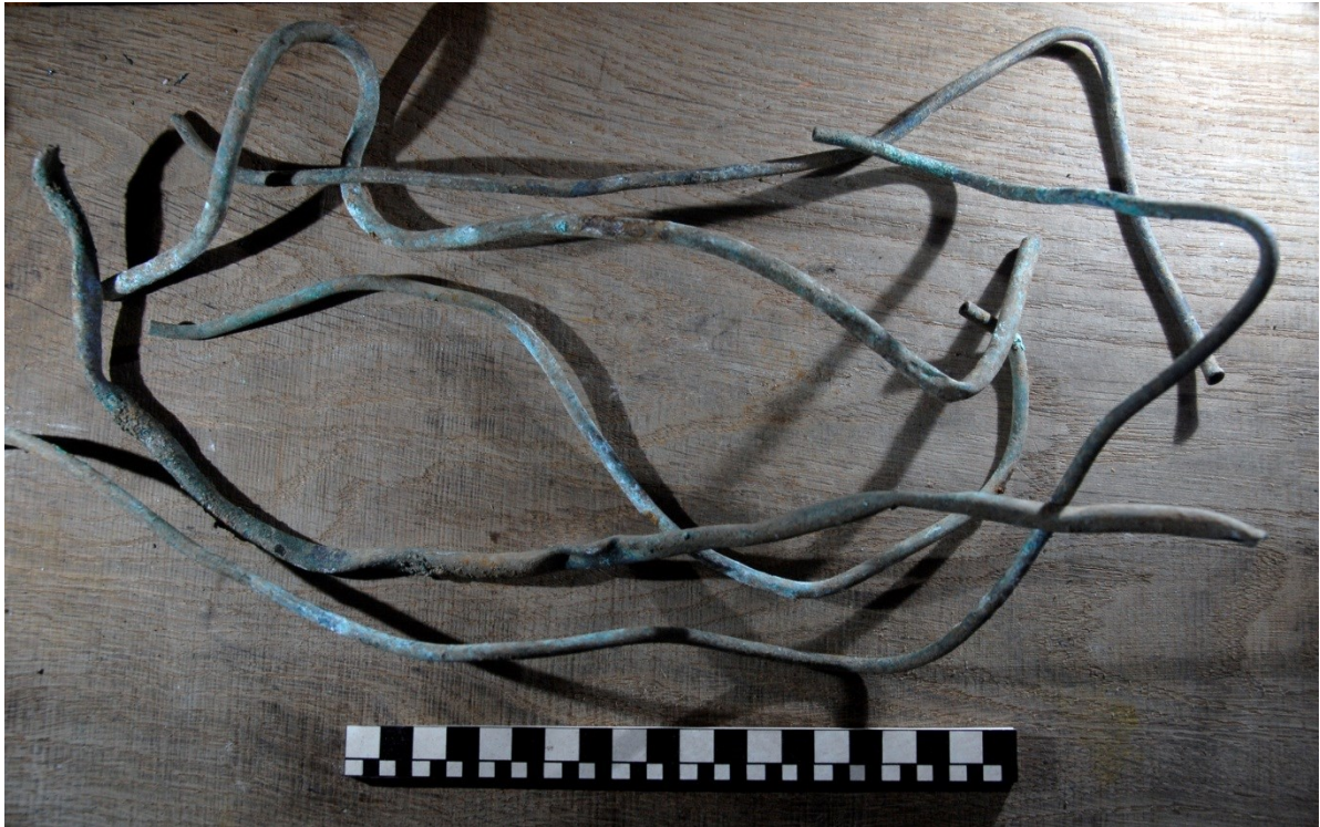
Fig 19. Sections of copper alloy hydraulic pipes associated with the undercarriage control system.
