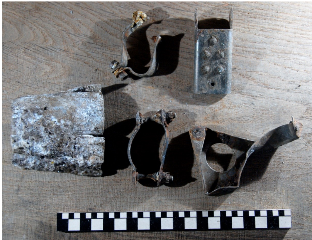
Fig 37. A large diameter aluminium pipe joiner, two Duralumin pipe clamps, a locking handle and a distinctively-shaped piece of Duralumin with a central eye.
