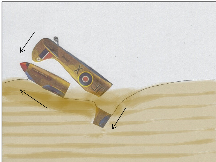
Fig 48. Crash stage 4. The engine block comes to rest (probably further on than shown here); the mid and tail section of fuselage may have ended up ahead of the impact crater as shown here, or standing more or less vertically on top of the crater as shown above; the fragmented remains of the mid cockpit area become buried at the base of the crater. Some above-ground parts of the aircraft wreckage are affected by fire. Above ground wreckage subsequently salvaged by the RAF maintenance unit team. The crater is partly backfilled.
