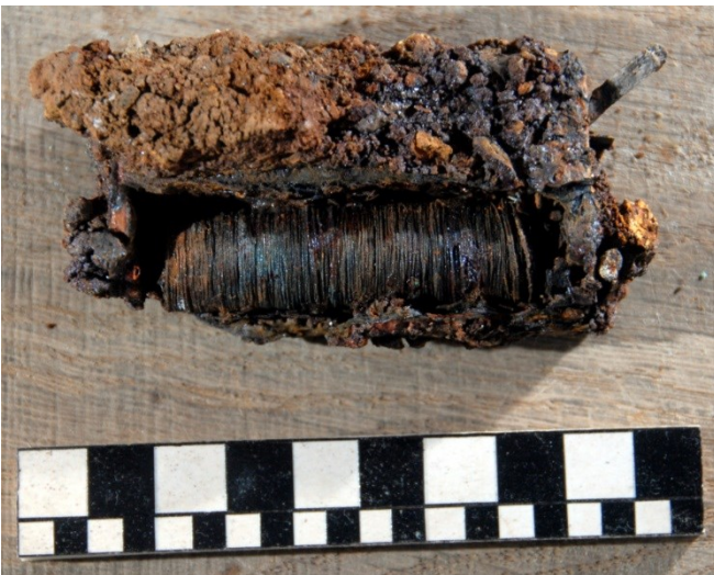
Fig 23. An electrical component consisting of two coils in a thin metal box.
