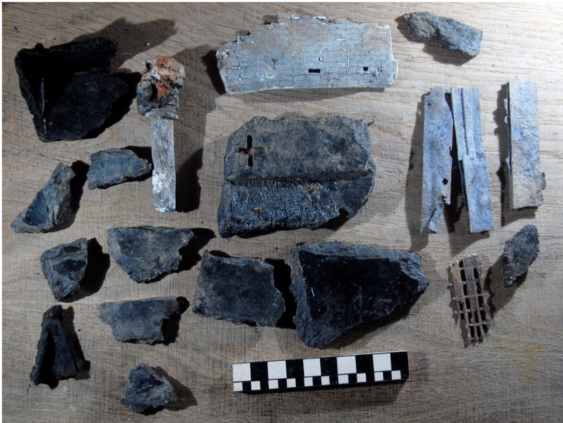
Fig 34. Fragments of the aircraft battery, including its casing, a terminal post, lead plates and separators.
