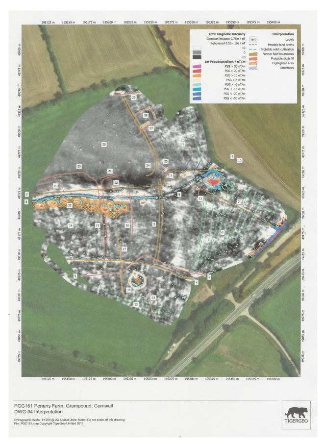
Fig 6. Interpreted geophysical survey results from Penans.
