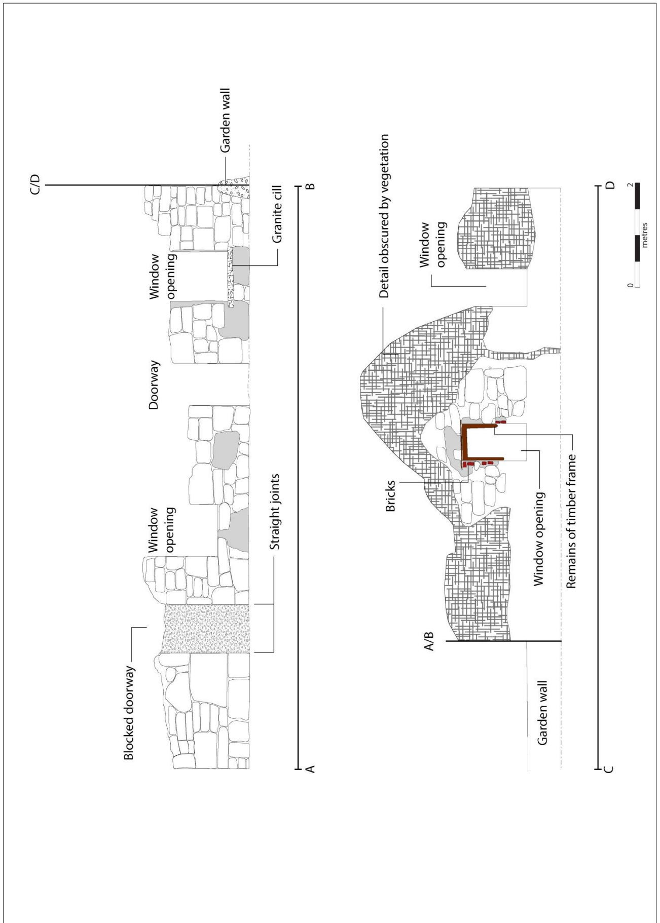
Figure 18. Field 4 Structure 2, Sections A-B and C-D.
