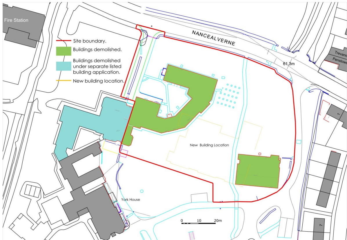
Figure 2. Site extent showing locations of demolished buildings and new building.
