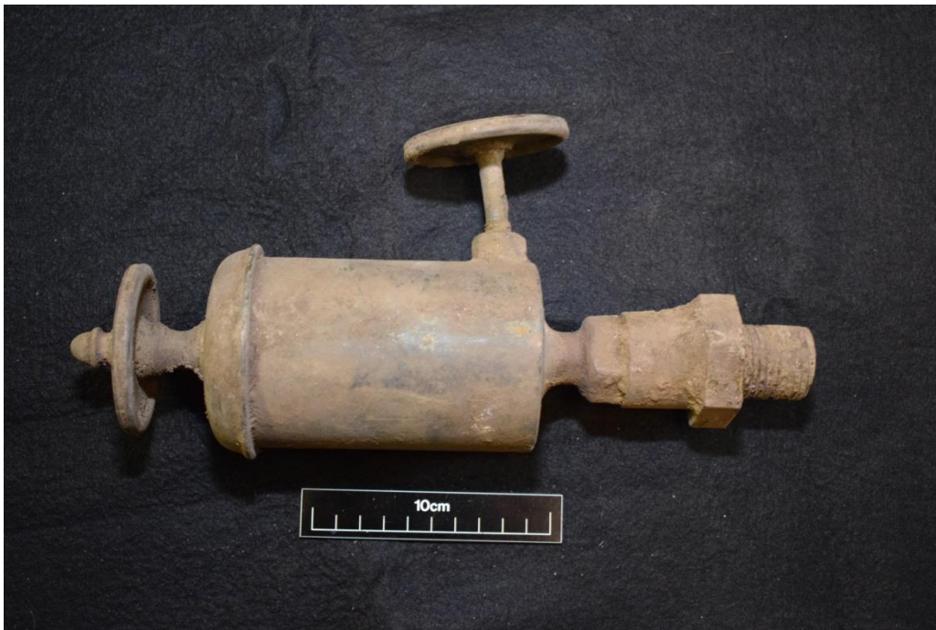
Figure 55: Lubricator from demolition rubble within the eastern boiler house.
