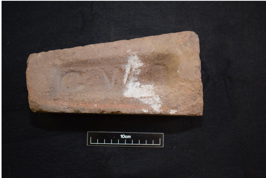
Figure 59: Chimney or side flue arch brick with 'GWR' stamp from the demolition rubble on the west side of the engine house.
