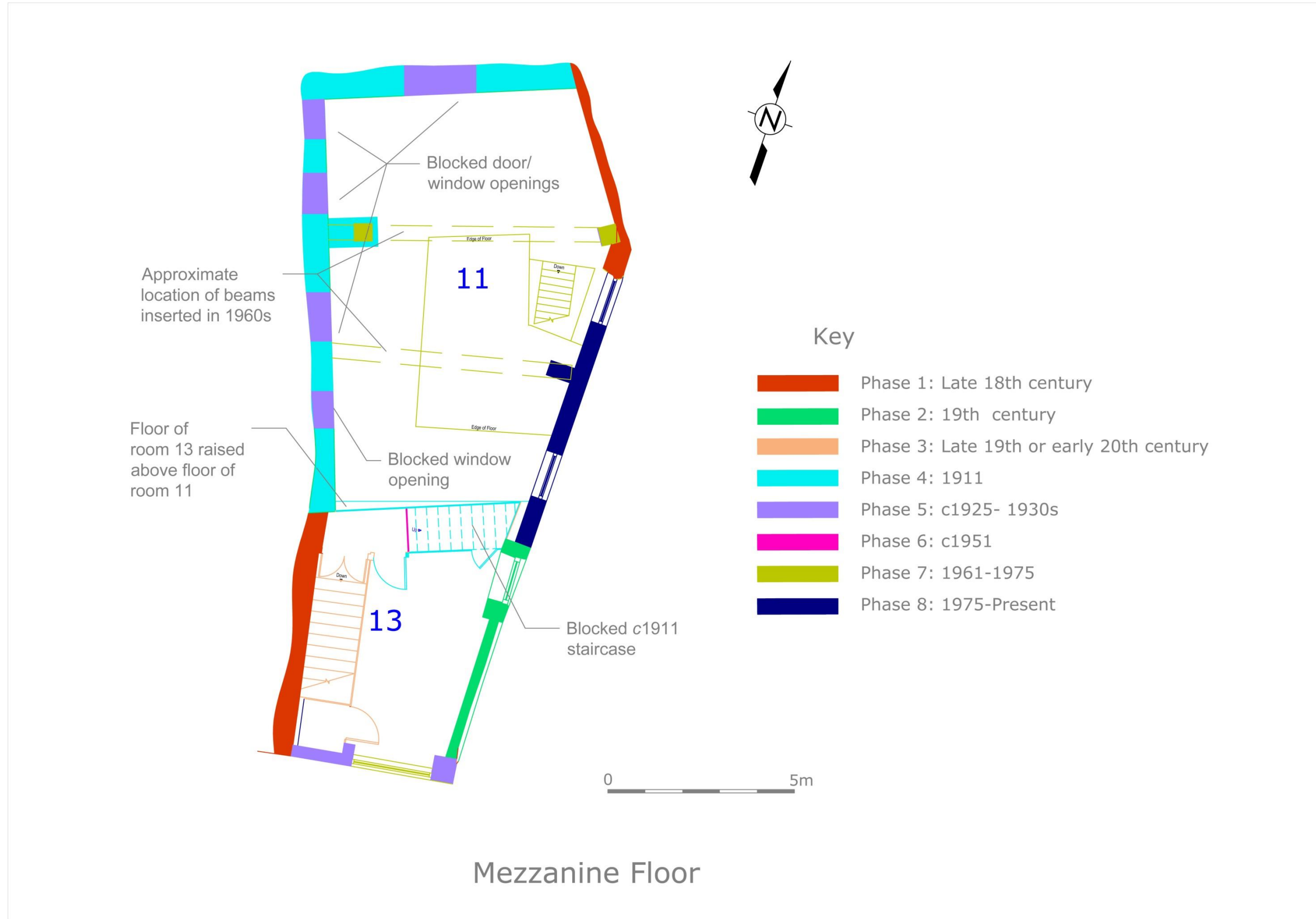
Fig 192 Mezzanine floor phase plan.
