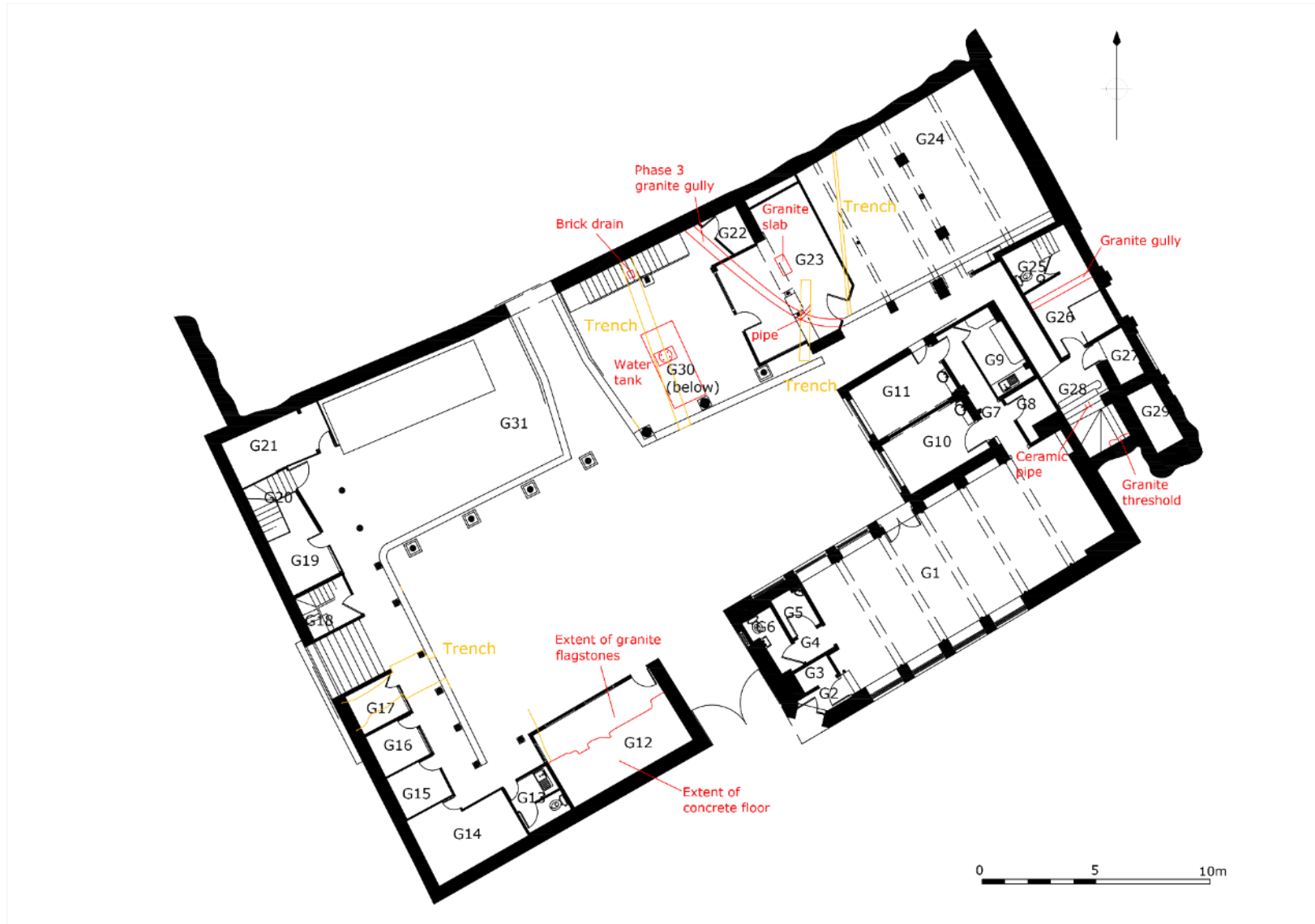
Fig 187 Location of trenches and features seen during the below-ground watching brief.
