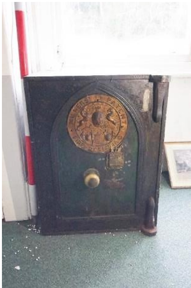
Fig 175 F17 safe 'Milner's patent fire resisting safe, powder proof solid lock Liverpool & London' from safe cupboard on north east wall.
