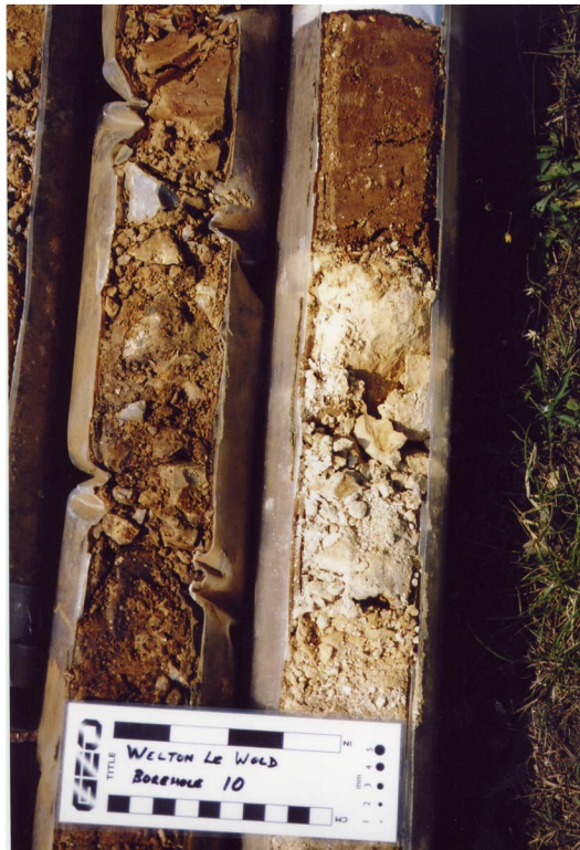
Plate 25: Core 10/4 showing concertina effect on the plastic sleeve
