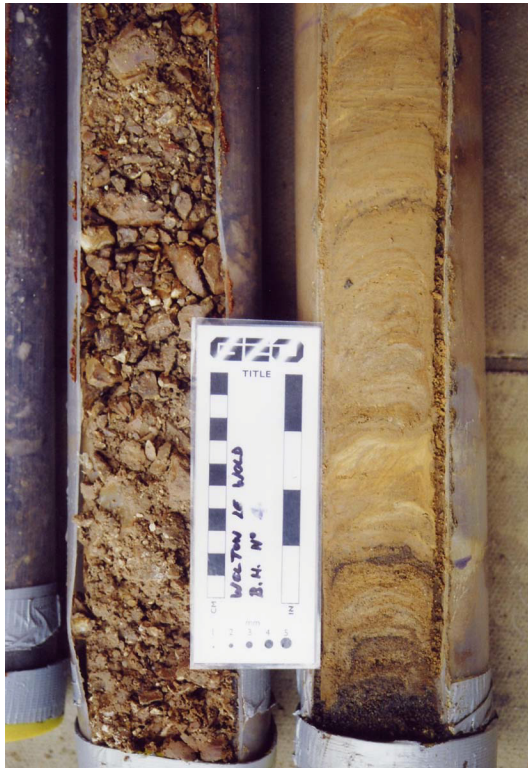
Plate 27: Core 4/2 showing drag effect of the fine grained sediments at the edge of the sleeve
