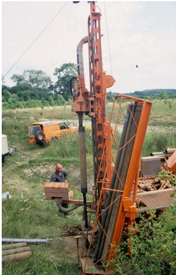
Plate 22: Driving the sampler in
