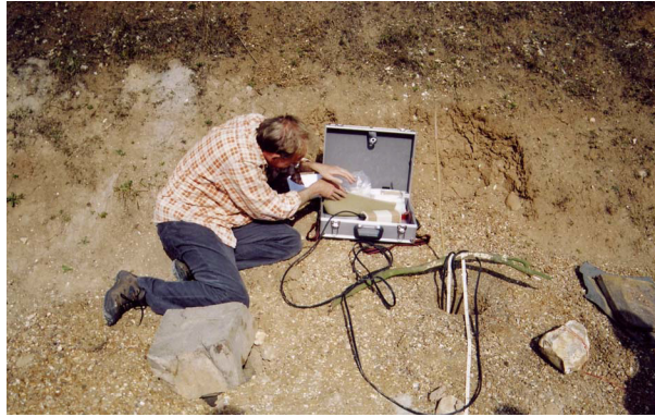
Plate 30: Jean-Luc measuring gamma spec. potential in Borehole 10A
