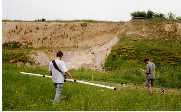
Plate 19: Ground Conductivity survey
