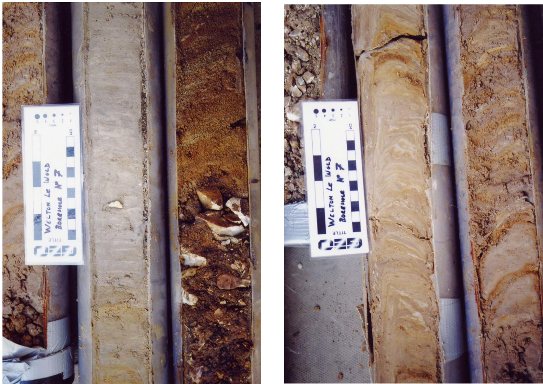
Plate 28: Cores 7/6 and 7/4 showing un-deformed and deformed laminates, the latter due to hydraulic power rather than the hammerhead action
