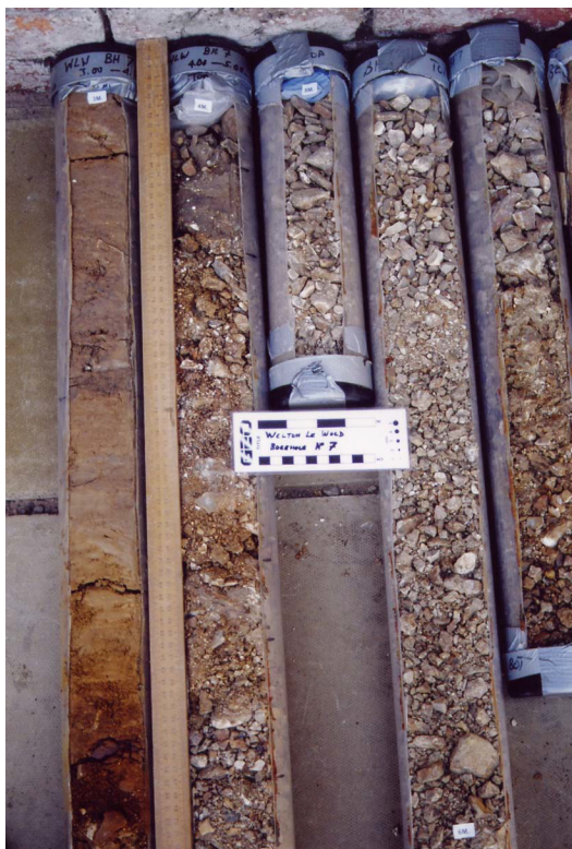
Plate 26: Core 7/3 showing shakedown of fine material in the upper 20 cm of the three right hand cores
