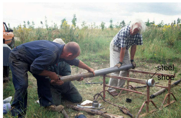
Plate 21: Plastic sleeve being extracted from the sampler
