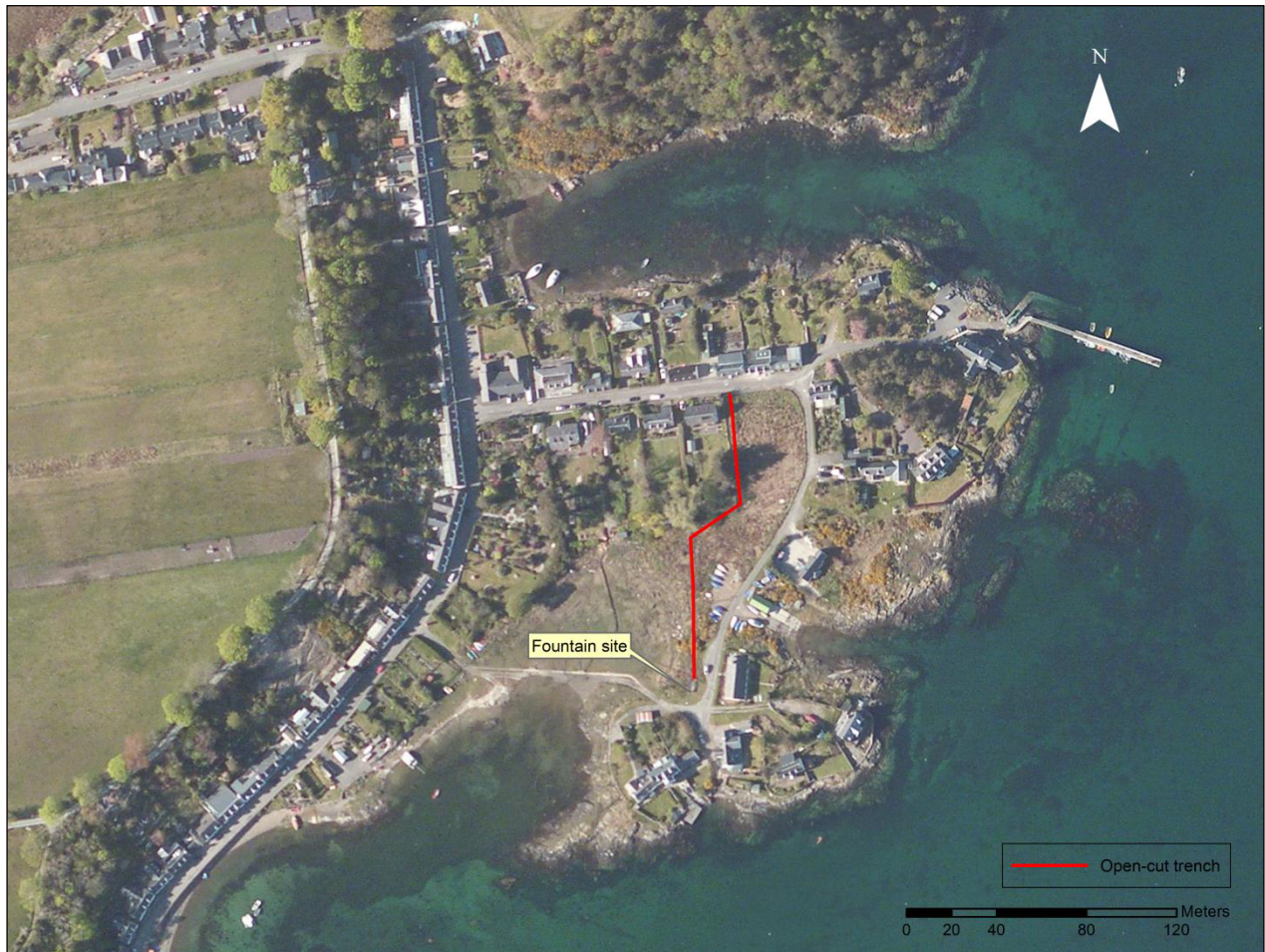
Figure 3 – Plockton water main renewal open-cut trench section
