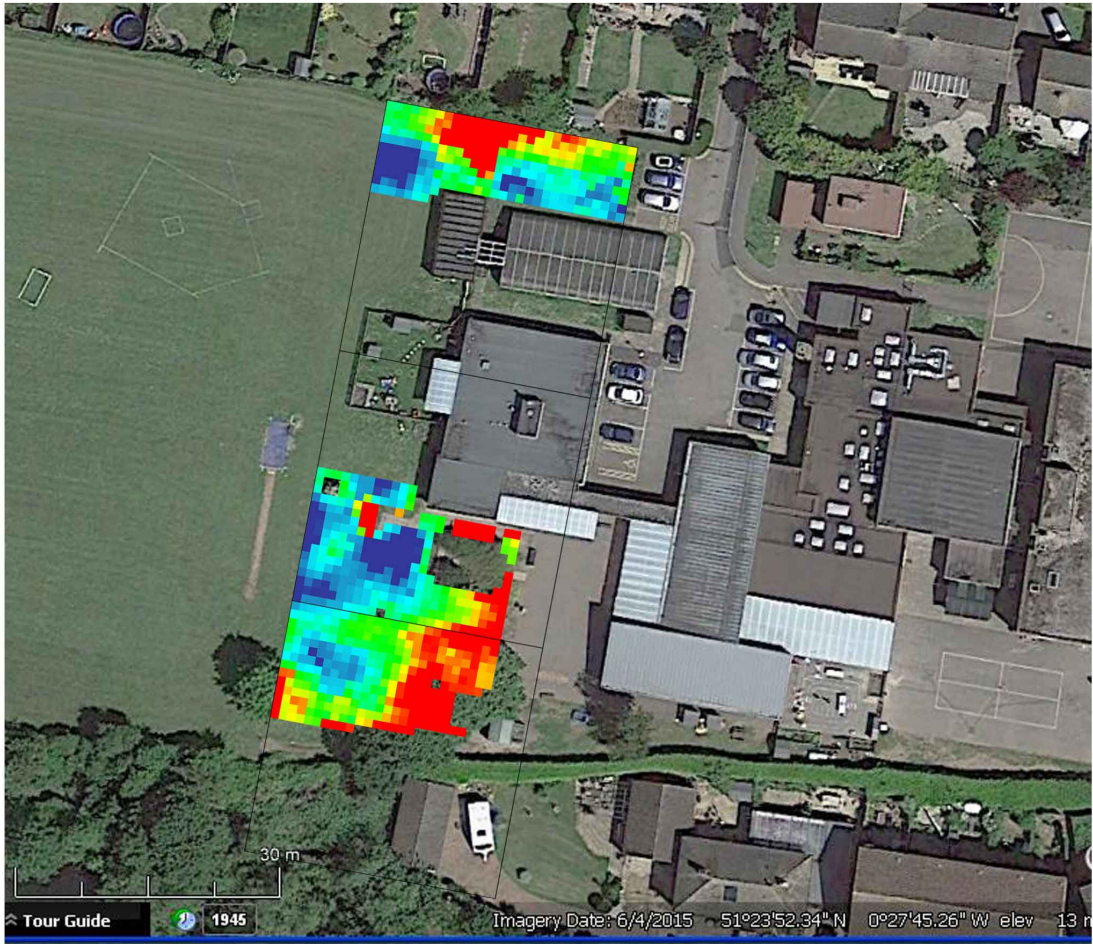
1 metre earth resistance on Google earth base
