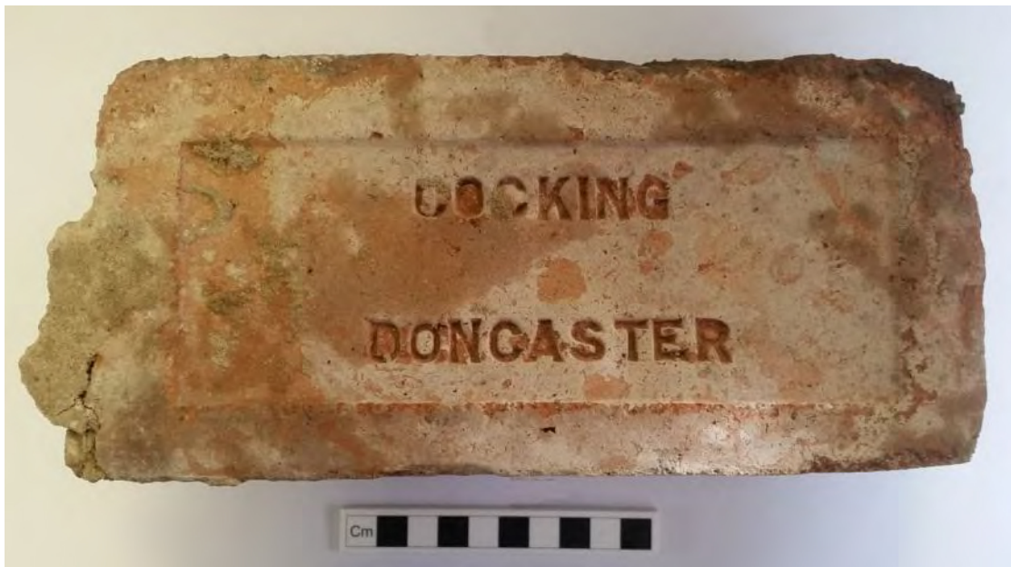
Plate 4: Example of the bricks used in the construction of the northern half of the building (Phase 2). Scale 10cm (1cm increments).
