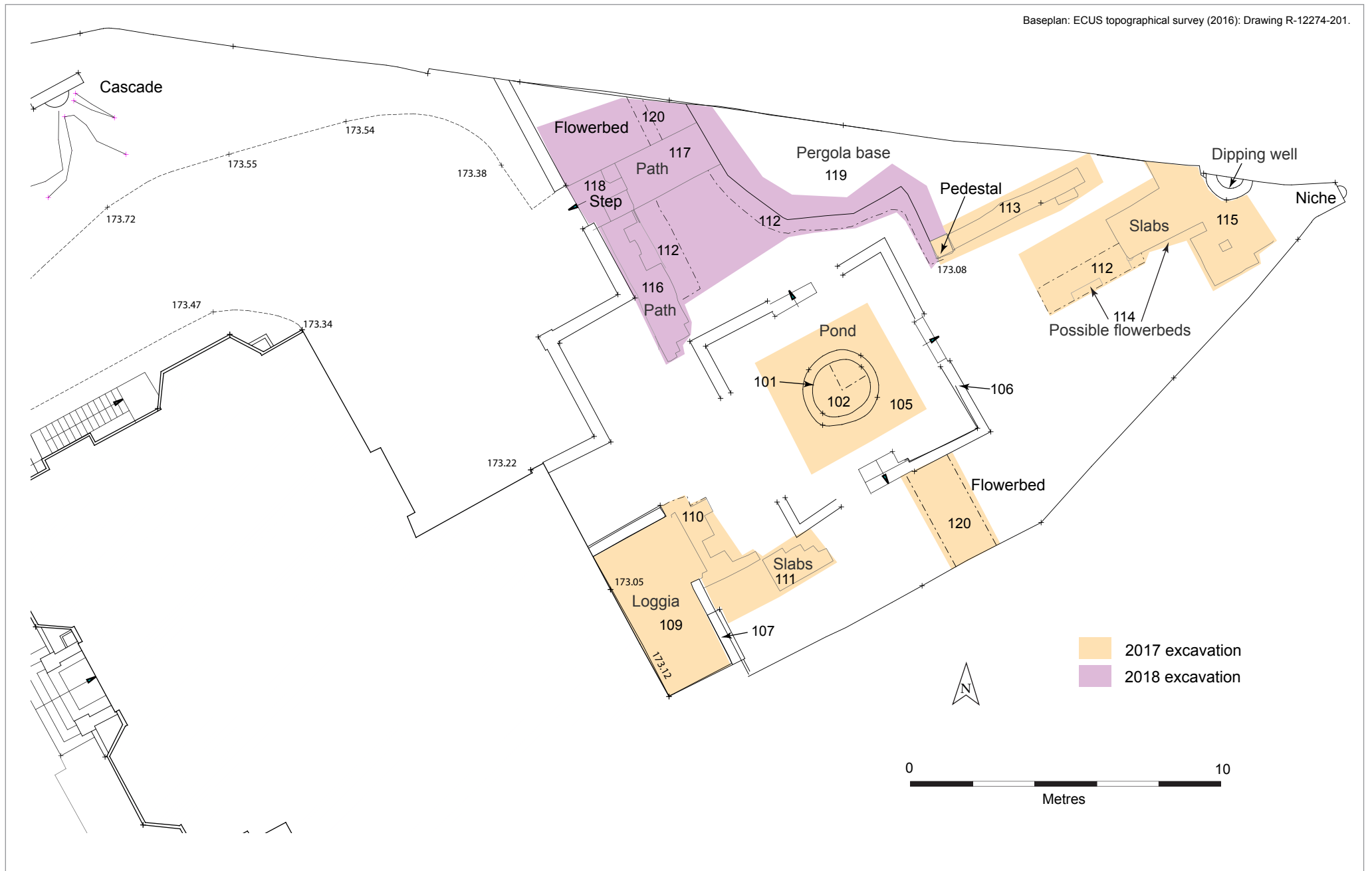
Figure 4: Broomhill Library: post-excavation plan
