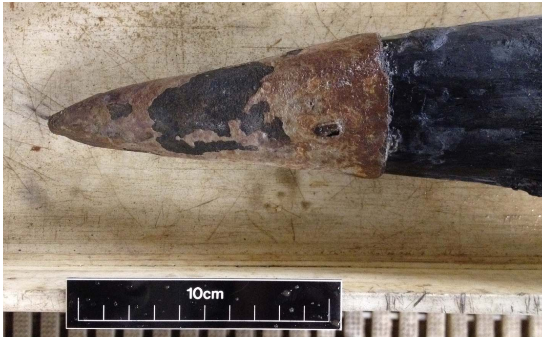
Plate 1. Fe shoe on tip of Pile (115) 2 of 2. Note nail hole 20mm from socket end showing as a dark rectangle. Scale 100mm (SJ Allen)
