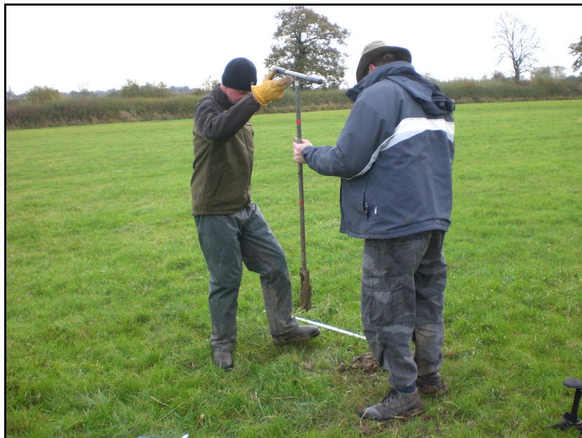
Figure 2. Sampling at Fen Meadow using an Eijelkamp silt shoe auger (Photo: J. Wheeler).
