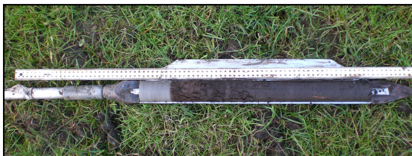
Figure 3. Russian chamber corer containing organic and alluvial sediments from Fen Meadow showing the erosive nature of the contact between two facies (Photo. J. Wheeler).
