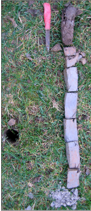
Figure 19. Soil profile in alluvium. Site 28: the alluvium is 79 cm thick over medium sand with stones.
