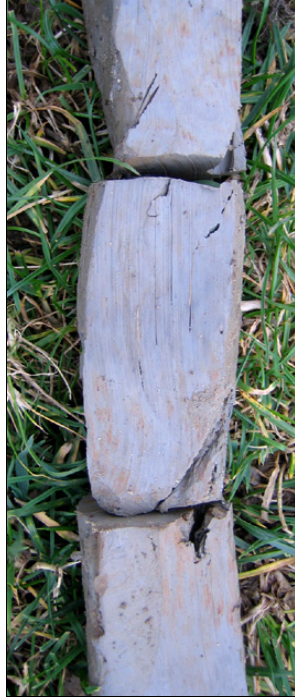
Figure 19. Soil profile in alluvium. Site 28: the alluvium is 79 cm thick over medium sand with stones.
