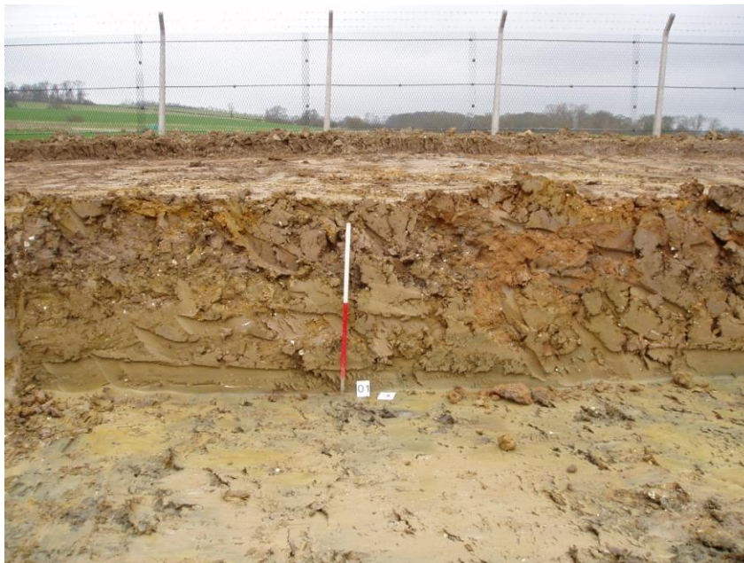
Plate 6 Area 02 depth of overburden (0002) shown overlying the boulder clay natural and clearly demonstrates the depth of made ground.
