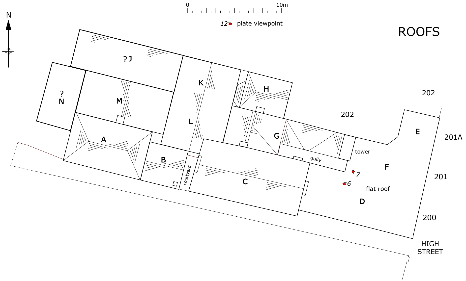
Figure 11: Plan of the roofs over Nos. 200 and 201 High Street, Lincoln. Skylights are not shown. Units are shown with codes A-N. Scale 1:200.
