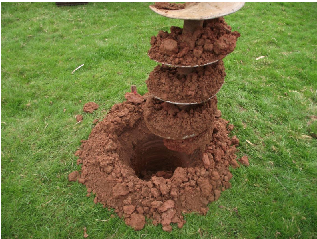
Plate 2. The auger bringing soils to the surface.
